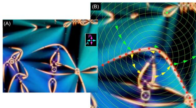
Fig. 2 Magnified images of parabolic focal-conic line and point defects in the freely suspended 2N/DIO film in the  $N_F$  phase shown in Fig. 1B. Two sets of circular contour lines, green and yellow, which the polarization/director field locally follows on opposite sides of the central parabola, are shown in (B). The parabolic focal-conic geometry guarantees that the director/polarization field, indicated schematically by colored arrows, is splay-free.
