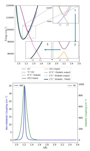
Fig. 7 Upper panel: Adiabatic and diabatic potential energy curves for CD' system. Lower panel: The NACs and DCs of the CD' system.
