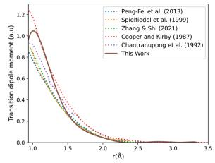
Fig. 3 CO  $A^1\Pi - X^1\Sigma^+$  transition dipole moment curves: ours compared to literature curves. 35,45,85,88
