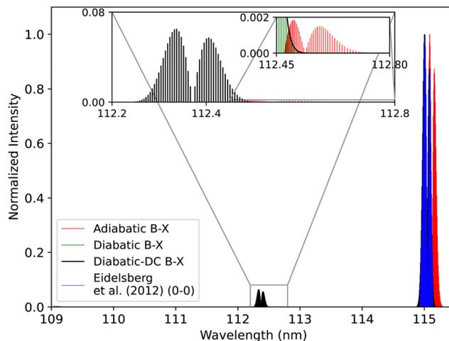
Fig. 18 Comparison between the adiabatic and diabatic representations of the  $B^1\Sigma^+-X^1\Sigma^+$  band system, and with Eidelsberg *et al.*<sup>112</sup> experiment.
