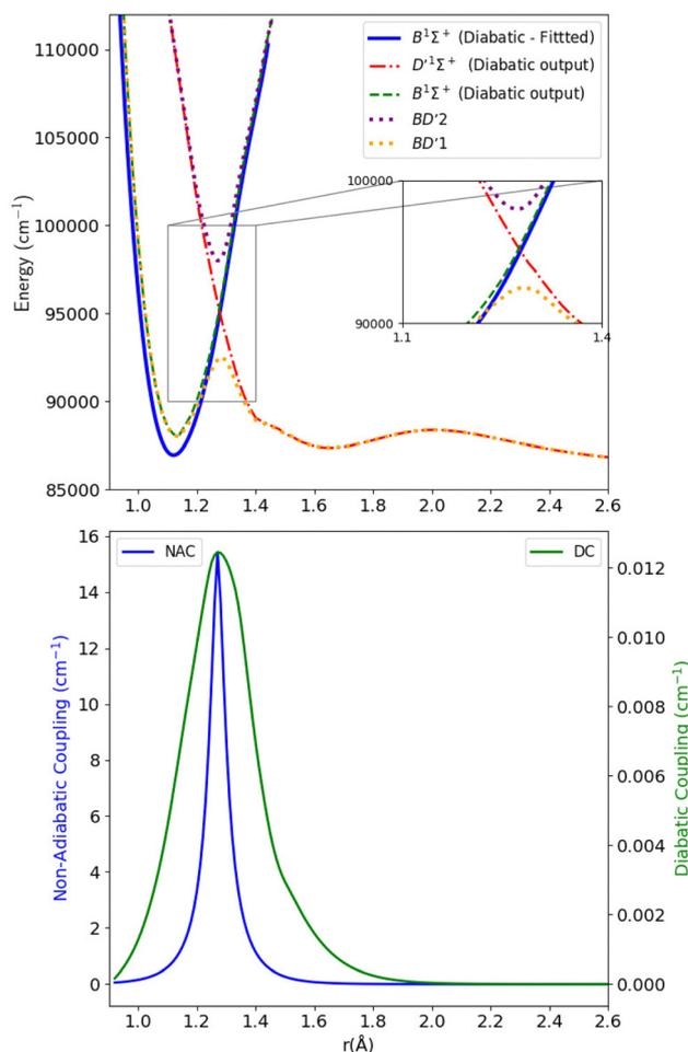
Fig. 5 Upper panel: Adiabatic and diabatic potential energy curves for the  $BD'$  system. Lower panel: The NACs and DCs of the  $BD'$  system.
