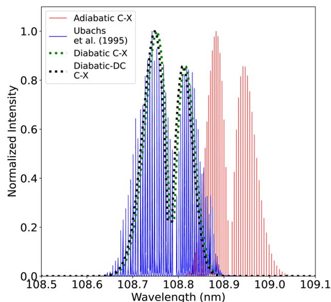
Fig. 21 Comparison between the adiabatic and diabatic representations of the (0-0)  $C^1\Sigma^+-X^1\Sigma^+$  band and with Ubachs *et al.*<sup>107</sup> experiment.
