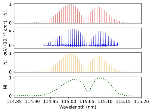
Fig. 12  $B^1\Sigma^+ - X^1\Sigma^+$  (0–0) spectrum: top panel, synthetic band calculated at Eidelsberg *et al.*<sup>41</sup> experimental conditions. Second panel, calibration (0–0) band due to Eidelsberg *et al.*<sup>41</sup> Third panel, synthetic band calculated at Federman *et al.*<sup>106</sup> experimental conditions. Bottom panel, (0–0) band due to Federman *et al.*<sup>106</sup> NI denotes normalized intensity.
