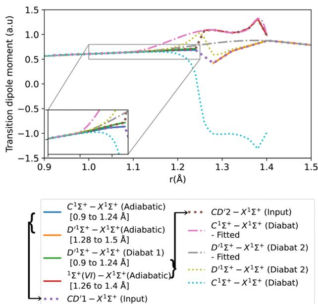
Fig. 8 Adiabatic and diabatic  $C^1\Sigma^+ - X^1\Sigma^+$  transition dipole moment curves.  $D^1\Sigma^+ - X^1\Sigma^+$  (Diabat 1) denotes the  $D^1\Sigma^+ - X^1\Sigma^+$  diabatic curve obtained from treating BD' system, and  $D^1\Sigma^+ - X^1\Sigma^+$  (Diabat 2) denotes the  $D^1\Sigma^+ - X^1\Sigma^+$  diabatic curve obtained from treating CD' system.
