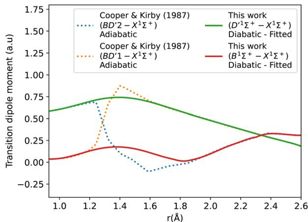
Fig. 6 Adiabatic and diabatic  $B^1\Sigma^+-X^1\Sigma^+$  transition dipole moment curves.
