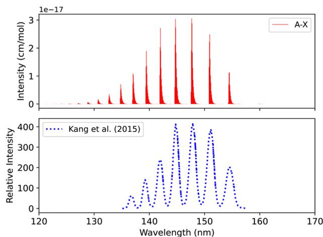
Fig. 9 Spectrum of  $A^1\Pi - X^1\Sigma^+$  band: upper plot, our calculation; lower plot, experiment of Kang et al.<sup>104</sup>
