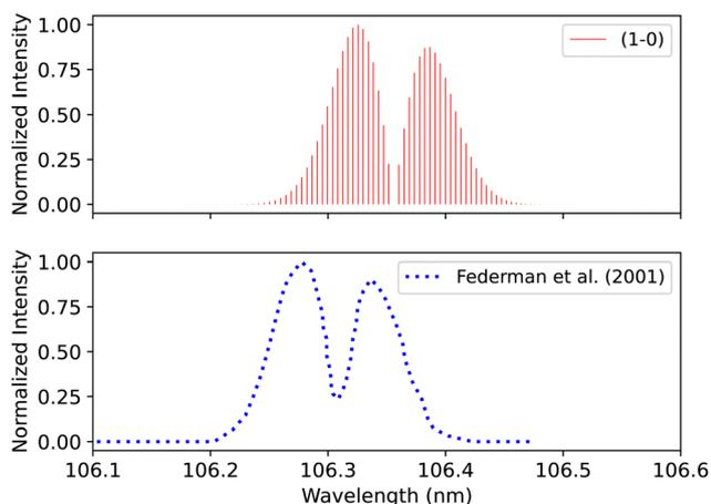
Fig. 15  $C^1\Sigma^+-X^1\Sigma^+$  (1–0) synthetic band compared with the (1–0) band measured by Federman *et al.*<sup>106</sup>
