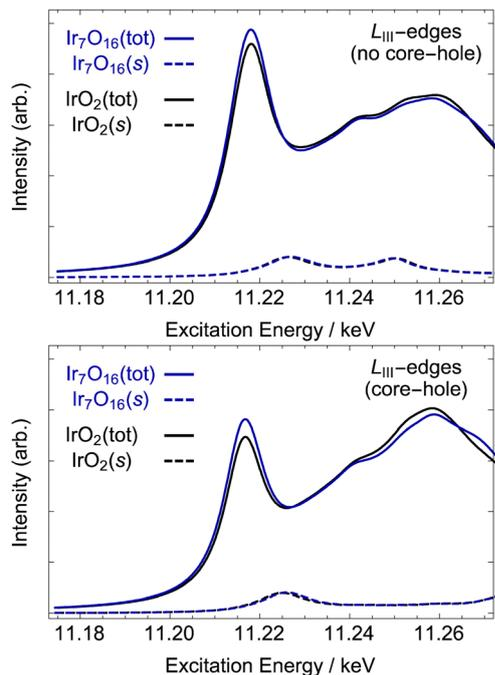
Fig. 6 Computed Ir  $L_{III}$ -edge without (top) and with (bottom) a 2p core-hole on the absorbing atom. The solid black curve shows the result for rutile-type  $IrO_2$ , and the blue curve shows the electron deficient iridium in the oxidized model compound  $Ir_7O_{16}$ , see methods. The two dashed line show the 6s contribution to each spectrum. See Fig. 1 for structural models.
