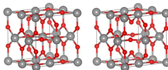
Fig. 1 The IrO<sub>2</sub> (left) and Ir<sub>7</sub>O<sub>16</sub> (right) super-cells used to model rutile-type IrO<sub>2</sub>. Iridium atoms are shown by way of grey spheres and oxygen red. Note the Ir vacancy in the centre of the Ir<sub>7</sub>O<sub>16</sub> cell.
