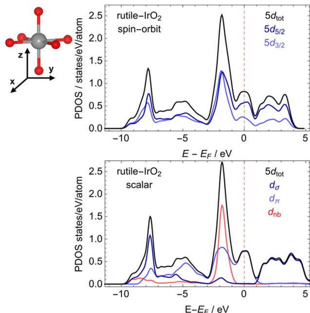
Fig. 5 PDOS of rutile-type  $\text{IrO}_2$  computed with (top) and without (bottom) spin-orbit coupling. In the scalar relativistic results, the 5d states are decomposed into  $\sigma$  - like ( $d_\sigma$ ),  $\pi$  - like ( $d_\pi$ ), and non-bonding ( $d_{nb}$ ) states. The geometry around a single  $\text{IrO}_6$  octahedron is also shown (top).
