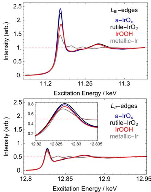
Fig. 2 Measured  $L_{III}$ -edges (top) and  $L_{II}$ -edges (bottom) of three compounds with known oxidation states, Ir metal (gray),  $\text{IrOOH}$  (red), and rutile-type- $\text{IrO}_2$  (black) along with that of amorphous- $\text{IrO}_x$  (blue). The dashed red lines show the normalized X-ray attenuation coefficients. The inset in  $L_{II}$ -edges shows the white line maxima.
