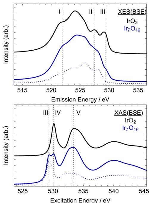
Fig. 7 Computed XE (top) and XA (bottom) O K-edge spectra of rutile-type  $IrO_2$  (black) and the oxidized model considered in ref. 5,  $Ir_7O_{16}$  (blue). The dotted blue line in the  $Ir_7O_{16}$  model shows the contribution from the electron-deficient oxygen referred to as  $O^{I-}$ . See Fig. 1 for structural models.
