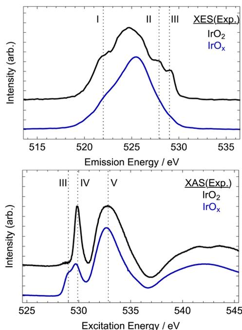
Fig. 8 Measured XE and XA O K-edge spectra of rutile-type  $\text{IrO}_2$  (top) and X-ray amorphous- $\text{IrO}_x$  (bottom), see also Fig. S1 (ESI<sup>†</sup>) for higher resolution XA spectra. See Fig. 1 for structural models.
