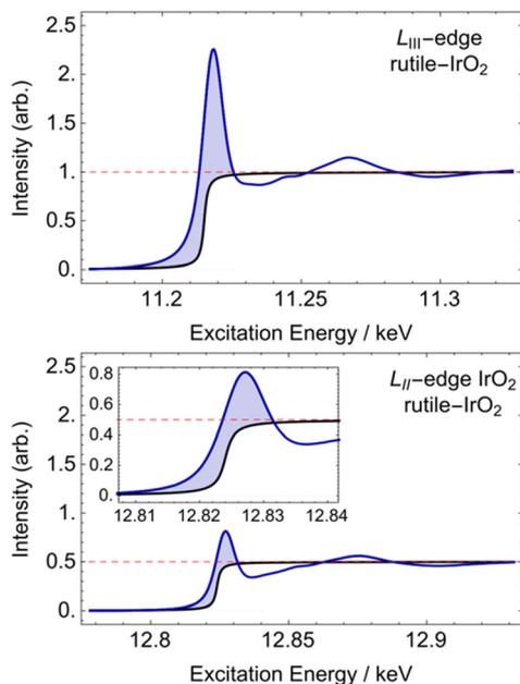
Fig. 3 The arctangent (black) used to model the continuum jump as described in the text shown using the rutile-type IrO<sub>2</sub> L<sub>III</sub>-edge (top) and L<sub>I</sub>-edge (bottom). The shaded region represents the contribution from the white-line. The inset in L<sub>I</sub>-edge shows the white line maximum.
