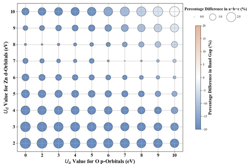
Fig. 7 Effect of Hubbard  $U$  values on rPBE band gap and lattice parameters of c-ZnO<sub>2</sub>.
