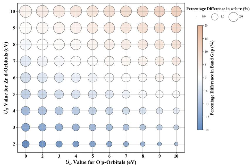
Fig. 9 Effect of Hubbard  $U$  values on rPBE band gap and lattice parameters of c-ZrO<sub>2</sub>.
