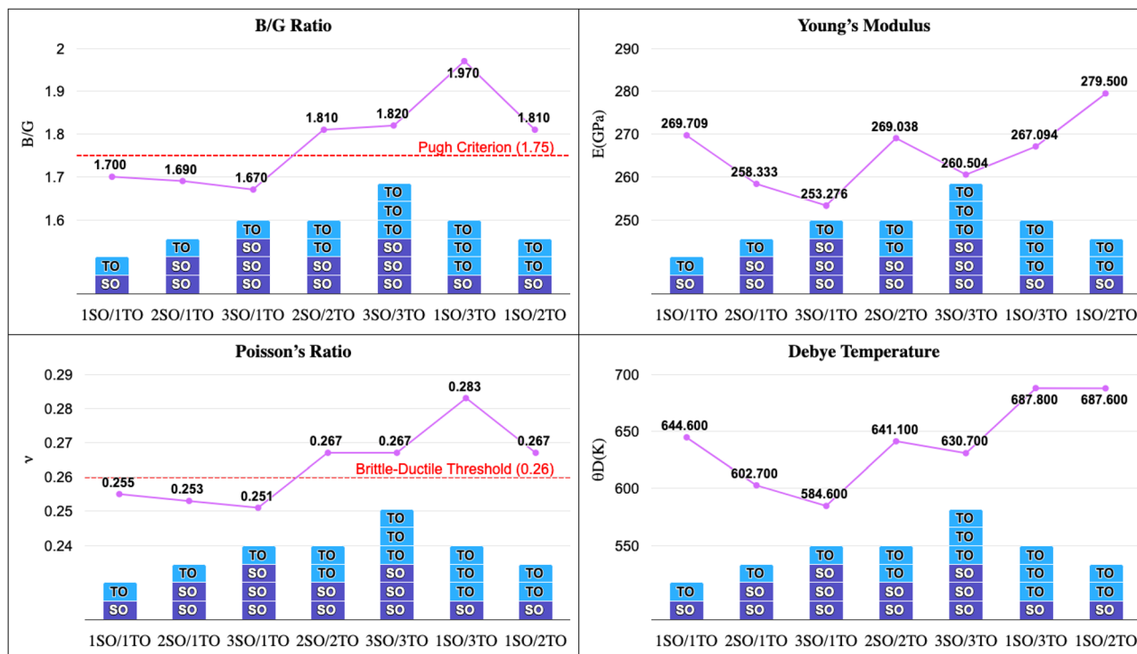
Fig. 6 Evolution of \frac{B}{G} ratio, Young's modulus ( E ), Poisson's ratio ( \nu ), and Debye temperature ( \theta_D ) of unstrained nSO/mTO superlattices for different ( n/m ) stacking periodicities.
