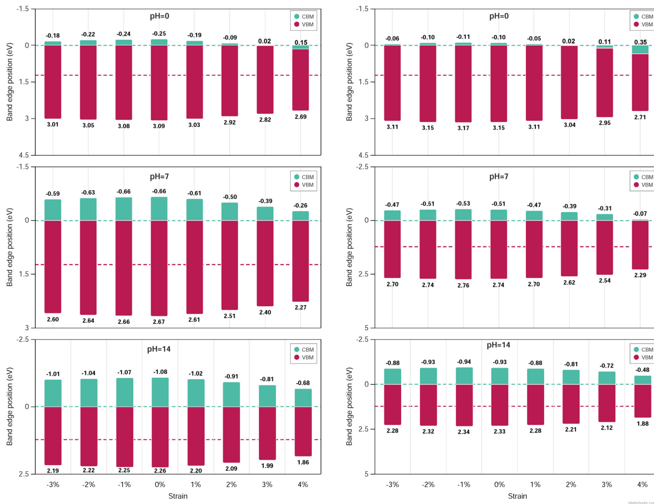
Fig. 14 Band edges alignment for 1SO/3TO (left) and 3SO/3TO (right) superlattices under biaxial tensile and compressive strains when pH equal 0 (upper part), 7 (middle part) and 14 (bottom part). The horizontal dashed lines are the water redox potentials.
