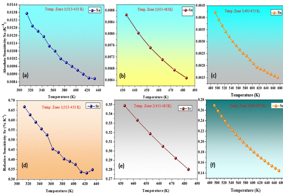
Fig. 7 The absolute sensitivities ( $S_a$ ) of the TCL pair,  $11\,655\text{ cm}^{-1}$  (858 nm) and  $11\,454\text{ cm}^{-1}$  (873 nm) in the three temperature regions in: (a) temp. zone 1 (313–433 K), (b) temp. zone 2 (443–483 K), and (c) temp. zone 3 (493–673 K), and the relative sensitivities ( $S_r$ ) in the three temperature regions in: (d) temp. zone 1, (e) temp. zone and (f) temp. zone 3, respectively.
