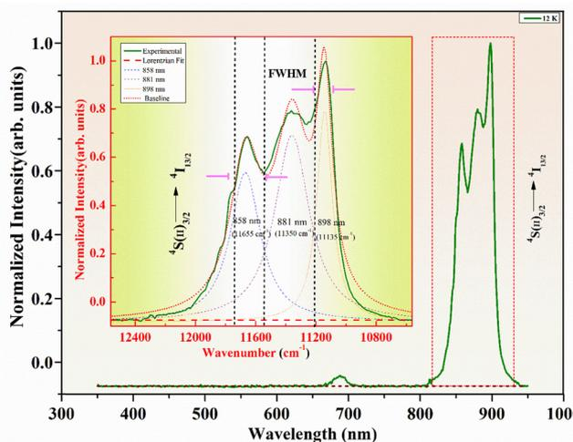
Fig. 2 UC emission spectra of the C1:PZT phosphor at 12 K, with 980 nm excitation. The zoomed red region displays the UC spectrum at 12 K within the range of 810–940 nm ( $12345\text{--}10638 \text{ cm}^{-1}$ ).
