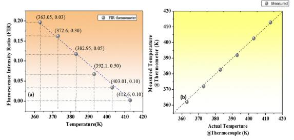
(a) Temperature measurements via the calibrated FIR curves; (b) temperature of electronic components using FIR and an infrared thermal imager.
