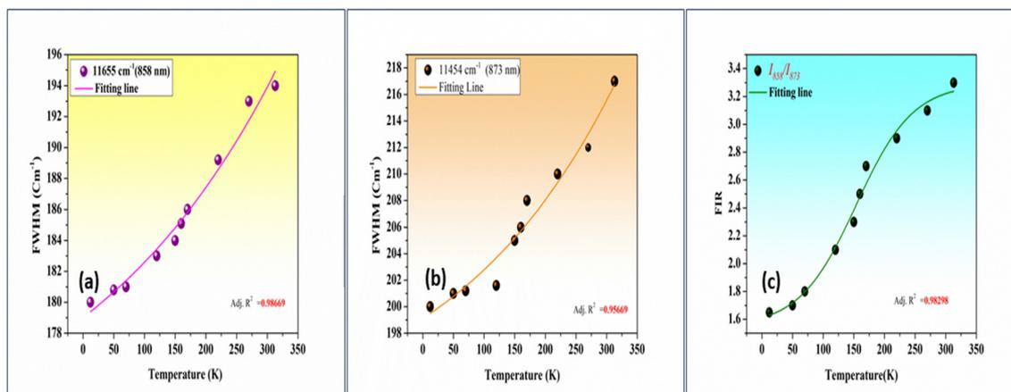
Fig. 4 The full width at half maximum (FWHM) of (a)  $11\,655 \text{ cm}^{-1}$  (858 nm) and (b)  $11\,454 \text{ cm}^{-1}$  (873 nm) bands as a function of temperature and (c) FIR of  $11\,655 \text{ cm}^{-1}$  (858 nm) and  $11\,454 \text{ cm}^{-1}$  (873 nm) emission bands as a function of temperature (cryogenic to room temperature).
