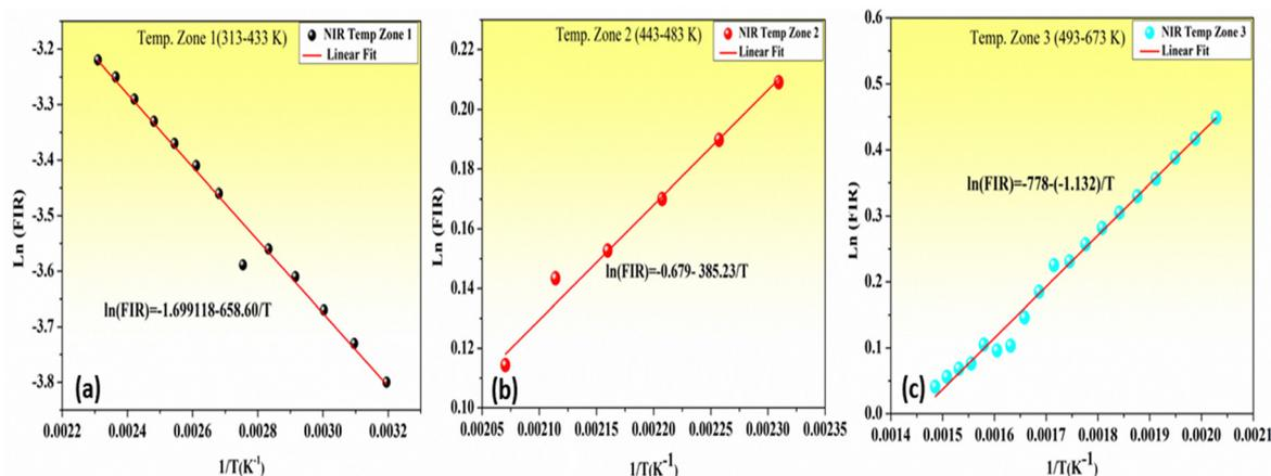
Fig. 6 Experimental and fitted FIR vs. temperature plots for the NIR emission in (a) temp. zone 1 (313–433 K), (b) temp. zone 2 (443–483 K), and (c) temp. zone 3 (493–673 K).
