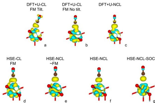
Fig. 7 Charge density difference calculated for all cases listed in Table 1. Yellow (light blue) isosurfaces correspond to positive (negative) differences. The isosurface value used in all cases is  $0.0034 e \text{ bohr}^{-3}$ . Brown spheres: carbon atom; red spheres: oxygen atom. Note the absence of charge accumulation around the carbon atom in the HSE-NCL and HSE-NCL-SOC cases.
