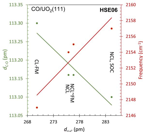
Fig. 9 A plot of the C to O bond distance ( $d_{\text{C-O}}$ ) (left y-axis) and its frequency (right y-axis) as a function of the bond distance with the surface ( $d_{\text{U-C}}$ ) as computed by HSE06 using the indicated methods. CL-FM: collinear ferromagnetic; NCL: non-collinear; SOC: spin-orbit coupling. The experimental  $\nu_{\text{CO}}$  frequency is equal to  $2160 \text{ cm}^{-1}$ .
