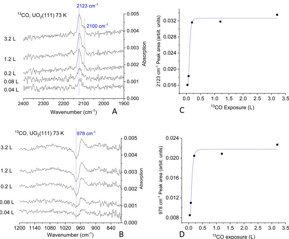
Fig. 3 Difference IRRAS spectra obtained after exposure of the clean  $\text{UO}_2(111)$  single crystal at 73 K at the indicated Langmuir exposure (one Langmuir =  $10^{-6}$  torr s). Effect of  $^{13}\text{CO}$  exposure on the surface uptake of  $\text{UO}_2(111)$  single crystal as tracked by the  $\nu^{13}\text{CO}$  peak at  $2123\text{ cm}^{-1}$  (A) and  $978\text{ cm}^{-1}$  peak (B). Note that both peaks saturate at the same exposure.
