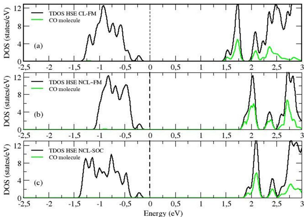
Fig. 8 The total density of state (TDOS, black line) of the CO adsorbed- $\text{UO}_2(111)$  system as computed by HSE06 together with the projected density of state on the molecular CO orbitals (green). (a) Collinear FM (HSE CL-FM) case, (b) non-collinear nearly FM (HSE NCL  $\sim$  FM) case, and (c) non-collinear with spin–orbit coupling (HSE NCL-SOC) case.
