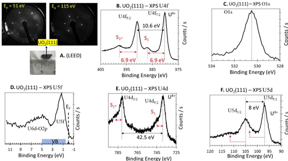
Fig. 1 Electron diffraction and photoelectron spectroscopy of  $\text{UO}_2(111)$  single crystal. (A) LEED at 51 and 115 eV primary excitation ( $E_p$ ); the sharp hexagonal spots at the given energy are in line with previous work (ref. 38) and indicate a (111) termination. (B) XPS U 4f. (C) XPS O 1s. (D) XPS valence band (U 5f, O 2p/U 6d). (E) XPS U 4d. (F) XPS U 5d.
