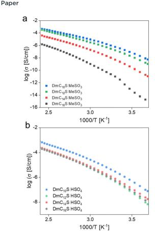
Fig. 11 Ionic conductivities of (a) mesylate based ILCs, and (b) hydrogensulfate based ILCs from room temperature to elevated temperatures.
