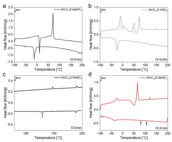
Fig. 4 2nd heating and cooling DSC runs for (a) DmC<sub>16</sub>S MeSO<sub>3</sub>, (b) DmC<sub>16</sub>S HSO<sub>4</sub>, and (c) DmC<sub>16</sub>S MeSO<sub>3</sub> with a heating/cooling rate of 5 K min<sup>-1</sup> (zoomed in to 80-200 °C), and (d) DmC<sub>14</sub>S MeSO<sub>3</sub>.
