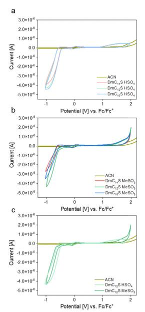
Fig. 10 Cyclic voltammograms of (a) hydrogensulfate based ILCs, (b) mesylate based ILCs, and (c) a comparison of DmC<sub>12</sub>S based ILCs.
