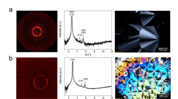
2θ [°] Fig. 7 Comparison of 2D diffraction patterns, diffractograms and POM images of C<sub>12</sub> based ILCs (a) DmC<sub>12</sub>S HSO<sub>4</sub> at 25 °C, and (b) DmC<sub>12</sub>S MeSO<sub>3</sub> at 20 °C.
