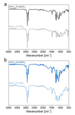
Fig. 2 Comparisons of the IR spectra of (a) DmC<sub>16</sub>S based ILCs and (b) DmC<sub>10</sub>S based ILCs.
