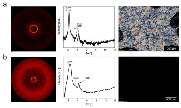
Fig. 6 Comparison of 2D diffraction patterns, integrated diffractograms and POM images for the two mesophases of DmC<sub>16</sub>S HSO<sub>4</sub> for (a) Col<sub>r</sub> at 45 °C and (b) Cub at 170 °C.
