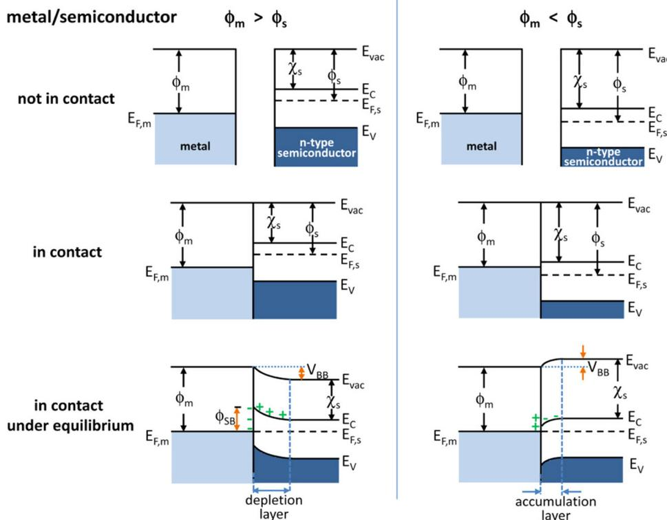
Fig. 1 Energy band diagrams of metal and n-type semiconductor contacts.  $E_{vac}$ , vacuum energy;  $E_C$ , energy of conduction band minimum;  $E_V$ , energy of valence band maximum;  $\phi_m$ , metal work function;  $\phi_s$ , semiconductor work function;  $\chi_s$ , electron affinity of the semiconductor.<sup>50</sup> Reprinted with permission from ref. 50. Copyright 2012 American Chemical Society.
