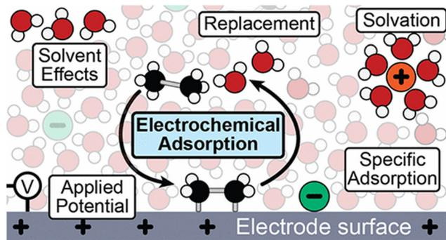
Fig. 8 Schematic of the electrochemical interface showing the interactions that must be considered in electrochemical adsorption processes. Not to scale.<sup>174</sup> Reprinted with permission from ref. 174. Copyright 2024 American Chemical Society.
