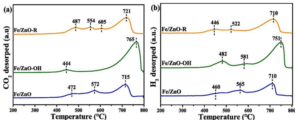
Fig. 4 CO<sub>2</sub>-TPD (a) and H<sub>2</sub>-TPD (b) profiles of CO-activated catalysts.<sup>152</sup> Reprinted with permission from ref. 152. Copyright 2024 Elsevier.
