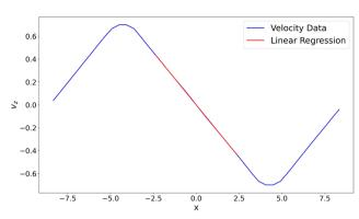
Fig. 3 Averaged velocity profile and corresponding linear regression in the middle area for the N-EQ Cross16 case with  $\Delta p_z = 0.01$ . The regions where the velocity gradient changes sign correspond to the position of the slabs.
