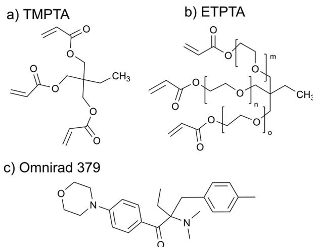
**Scheme 1** Chemical structures of the monomers (a) trimethylolpropane triacrylate (TMPTA), (b) ethoxylated trimethylolpropane triacrylate (ETPTA) and (c) the photoinitiator 2-(dimethylamino)-2-(4-methylbenzyl)-1-(4-morpholinophenyl)butan-1-one (Omnirad 379). The average molecular weight of ETPTA is 428, which corresponds to an average  $m$ ,  $n$ ,  $o = 1$ .
