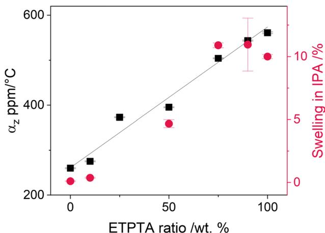
Fig. 2 Linear thermal expansion coefficient in z-direction  $\alpha_z$  in the temperature range 80–120 °C and thickness swelling in IPA for p(TMPTA–ETPTA) thin films as a function of ETPTA mixing ratio. The black line corresponds to the linear fit of the thermal expansion coefficient.
