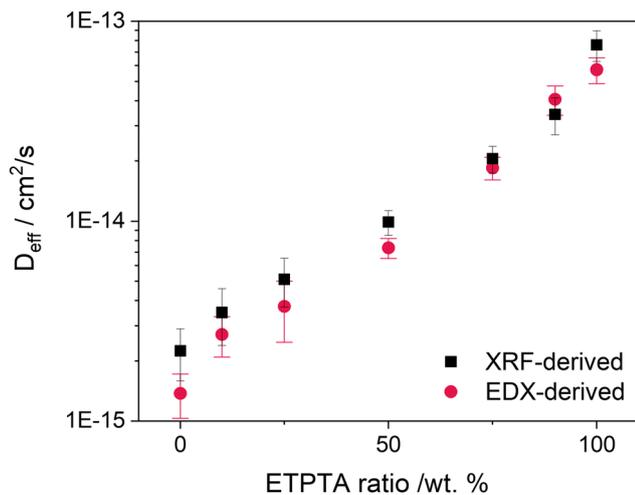
Fig. 6 Estimates for the effective diffusion coefficient  $D_{\text{eff}}$  for the different p(TMPTA–ETPTA) copolymer compositions at 120 °C calculated by linear fitting of the normalized temporal Zn uptake measured by XRF and EDX (Fig. S9, ESI†) according to eqn (1).
