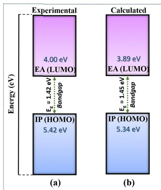
Fig. 3 (a) Electron affinity (EA), ionization potential (IP) and bandgap of the NDI-TVT polymer taken from experimental data of Kim *et al.*<sup>26</sup> (b) Calculated IP, EA and bandgap of the NDI-TVT polymer in the solvent phase.
