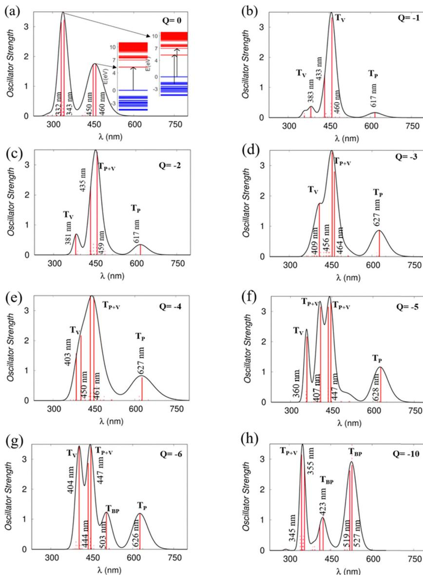
Fig. 7 UV vis/NIR absorption spectra of (a) the charge neutral PNDI-TVT chain and (b)–(h) the doped PNDI-TVT chain at various charged states from  $Q = -1$  to  $-6$  and  $-10$  indicating the corresponding electronic transitions calculated in the solvent phase.
