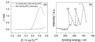
Fig. 2 (a) LSV traces from OCP to 0.7 V vs.  $Fc^{0/+}$  with 10 mM Bu<sub>4</sub>NCl (red) and without (black) chloride in 500 mM Bu<sub>4</sub>NPF<sub>6</sub> supporting electrolyte; (b) Cl 2p XPS of the GC carbon electrode after the LSV experiment showing both  $Cl^-$  and oxidized  $Cl^0$ .
