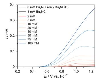
Fig. 3 LSV curves on a GC disk in solutions of varying chloride concentration. The scan rate is 5 mV  $\rm s^{-1}$ . The control experiment with no chloride is also included (gray) for comparison.
