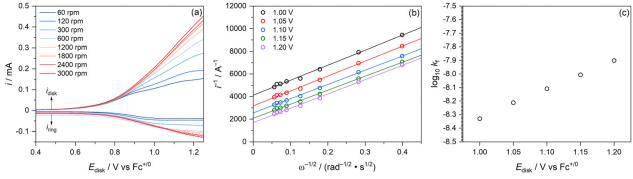
Fig. 5 (a) RRDE LSV ( $i-E_{disk}$ ) with a GC disk and Pt ring in 5 mM Bu<sub>4</sub>NCl and 100 mM Bu<sub>4</sub>NOTf electrolyte in EtOH solvent. The scan rate is 20 mV s<sup>-1</sup> and  $E_{ring}$  is poised at -0.4 V vs.  $Fc^{+/0}$ . The cell is sparged with argon prior to recording the data; (b) K–L plot of the LSV data; (c) trend in kinetic rate constant determined from the kinetic current as a function of disk potential.
