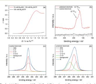
Fig. 1 (a) LSV sweep of 10 mM Bu<sub>4</sub>NCl in ethanol. The scan rate is 1 mV s<sup>-1</sup>; XPS data on GC electrodes. (b) Cl 2p after soaking or polarizing in Bu<sub>4</sub>NCl in ethanol solvent; (c) C 1s after soaking; (d) C 1s after polarizing
