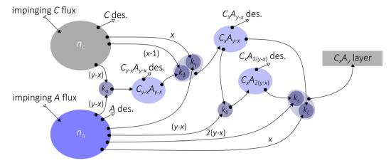
Fig. 5 MBE reaction scheme for binary III-VI and IV-VI materials, showing impinging  $\phi_c$  and  $\phi_a$ , resulting cation  $n_c$ , anion  $n_a$ , respective subcompound reservoirs, and the final compound  $C_xA_v$ . Chemical reactions (12)–(17) are indicated by reaction rate constants  $k_i$ .
