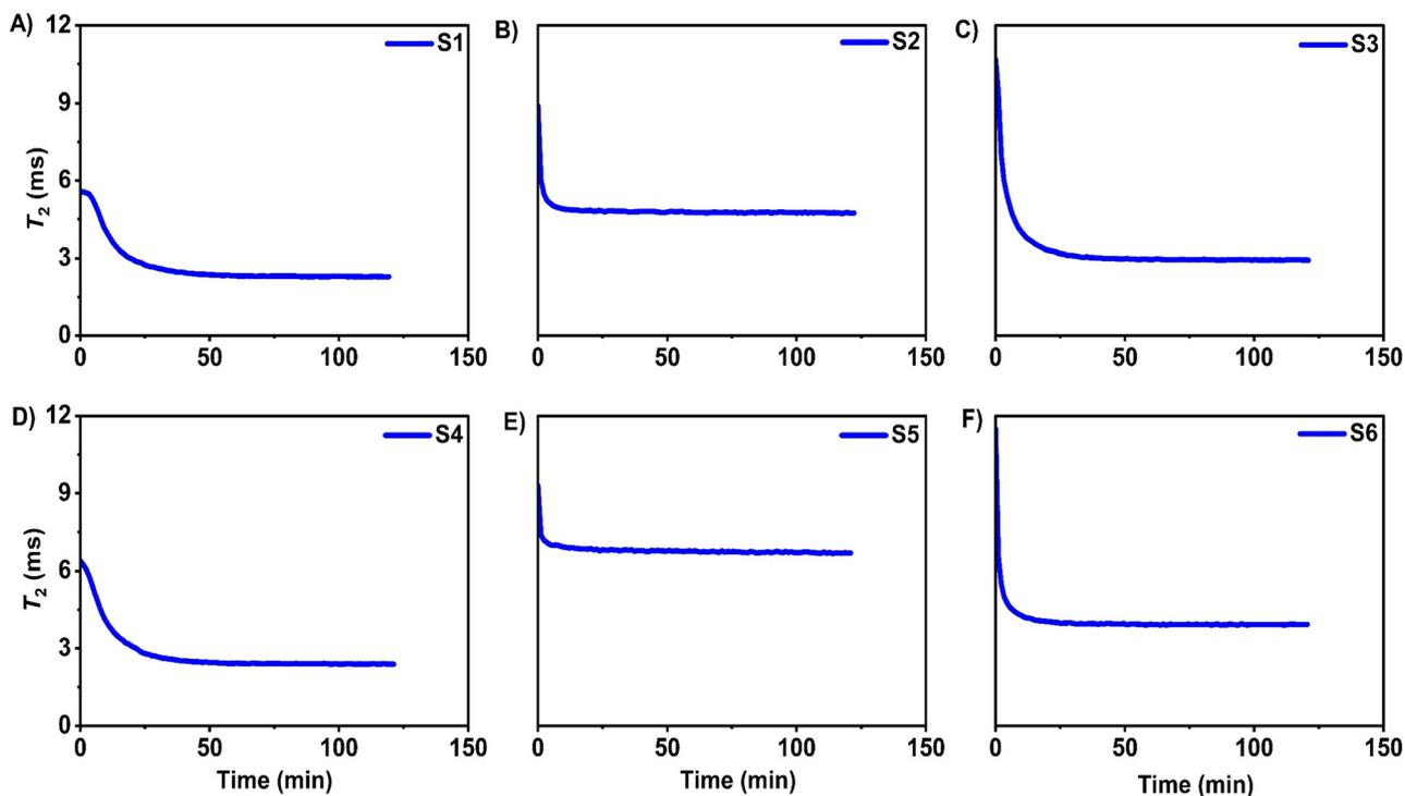
Fig. 13  $T_2$  relaxation times measured during short-term sedimentation experiments (A)–(F) for samples S1 to S6, respectively. The displayed curves illustrate decreasing  $T_2$  relaxation times, which indicate a transition from free to more confined water states within the sediment.
