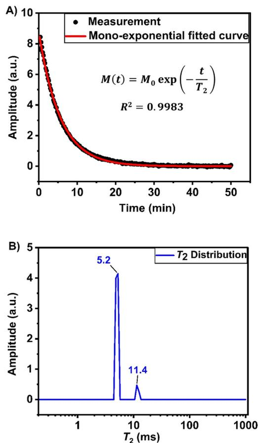
Fig. 9 (A)  $T_2$  decay curve measured in a typical CPMG experiment with sample S1, along with its mono-exponential fit. The close agreement between the measured data (black dots) and the fitted curve (red line) demonstrates the suitability of the mono-exponential model. (B) Relaxation time distribution obtained using the Laplace inversion procedure, showing two distinct components at 5.2 ms (dominant) and 11.4 ms (minor).
