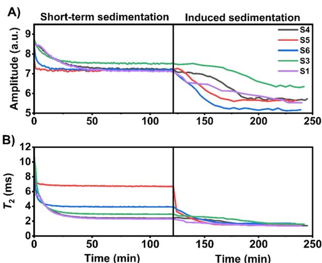
Fig. 14 Comparative analysis of echo amplitudes (A) and  $T_2$  relaxation times (B) for samples S1 and S3–S6 during the short-term sedimentation and subsequent gentle shaking. The left panels show the initial sedimentation phase, highlighting rapid changes in both parameters, while the right panels illustrate the impact of mechanical shaking, marked by further reductions in amplitude and  $T_2$  relaxation, indicating enhanced sediment compaction and water confinement.
