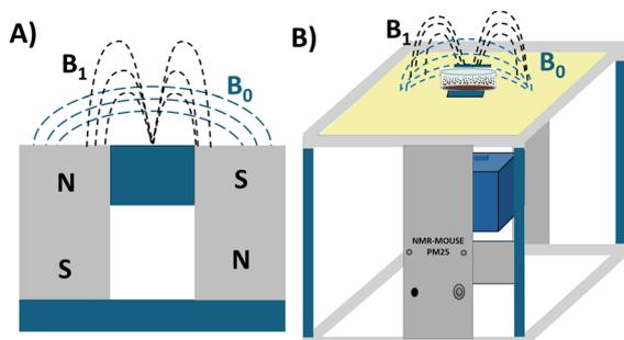
**Fig. 1** (A) Schematic of NMR-MOUSE PM25 used in this study. The device features a permanent magnet in conjunction with a surface RF coil to generate static  $B_0$  and oscillating  $B_1$  magnetic fields, respectively, enabling localized, non-invasive  $^1\text{H}$  NMR measurements of water content in near-surface regions.<sup>25–28</sup> (B) NMR-MOUSE PM25 device mounted on a lift for vertical sample profiling of a tailings sample.
