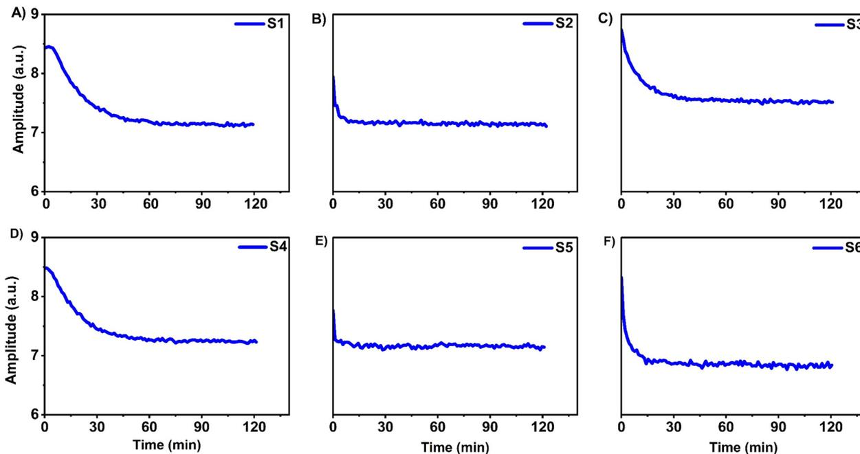
Fig. 12 Experimental  $^1\text{H}$  NMR signal amplitudes measured during the short-term sedimentation experiments as a function of time (A)–(F) for the samples from S1 to S6, respectively. All curves demonstrated an initial rapid decrease, followed by stabilization in echo amplitude across different samples.
