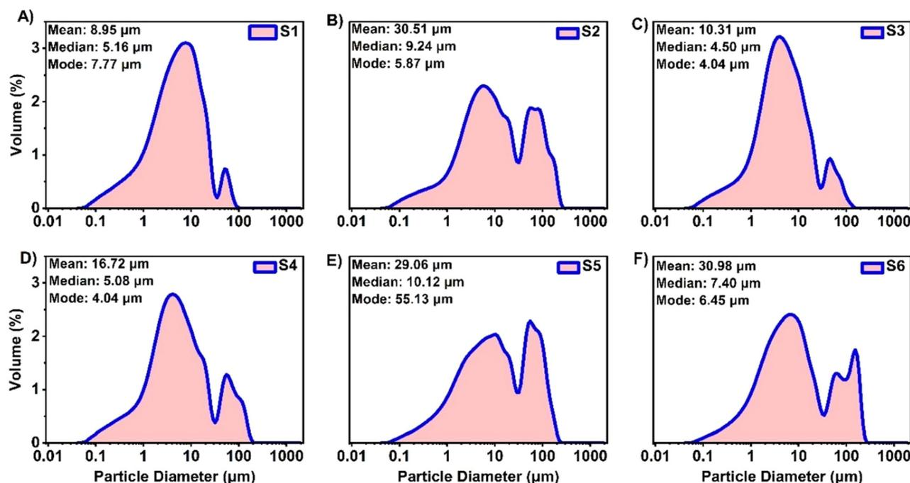
Fig. 4 Particle-size distribution (PSD) graphs for samples S1 to S6 (A)–(F), respectively, illustrating a broad range of particle diameters with specific mean, median, and mode values for each sample. These distributions highlight the variability in particle size across different locations within the tailings storage facility.
