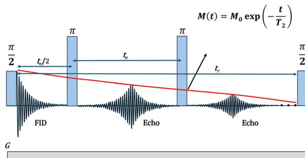
**Fig. 2** CPMG NMR pulse sequence diagram, illustrating the signal acquisition and measurement of  $T_2$  relaxation times using NMR-MOUSE during sedimentation and drying experiments.  $M(t)$  represents the total magnetization of the sample at the echo maxima at time  $t$  after the initial  $\pi/2$ -pulse.  $M_0$  is the initial magnetization, and  $T_2$  is the transverse relaxation time.
