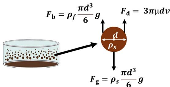
Fig. 7 Forces acting on a spherical particle, including fluid gravitational  $F_g$ , buoyancy  $F_b$ , and drag  $F_d$  forces. Together, they determine the particles' settling velocity under laminar flow conditions.
