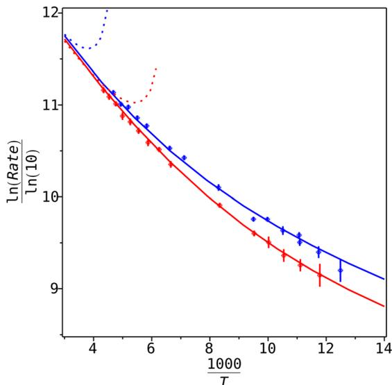
Fig. 1 Comparison of experimental<sup>34</sup> and theoretical hopping rates for H and D on Pt(111). Data for H are colored blue, for D red. The solid lines are the theoretical result based on eqn (24), the dotted lines are obtained with the parabolic barrier theory (eqn (7)).
