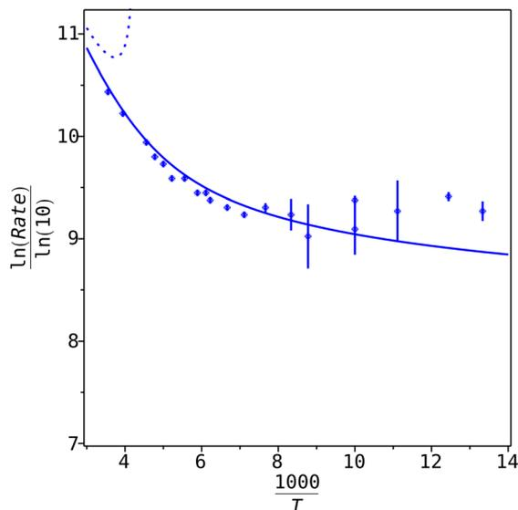
Fig. 2 Comparison of experimental<sup>22</sup> and theoretical hopping rates for H on Ru(0001). The solid line is the theoretical result based on eqn (24), the dotted line shows the parabolic barrier theory result (eqn (7)).
