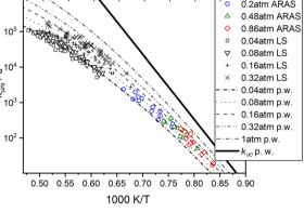
Fig. 6 Fall-off first-order Arrhenius results for  $k_2$ . Color symbols are  $k_2$ from ARAS experiments; Black symbols are  $k_2$  from LS experiments; Lines are theoretical predictions from this work. The lower plot is zoomed to the experimental data
