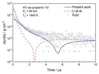
**Fig. 4** Typical experimental results (symbols) for absolute density gradients and comparison with model predictions (lines). The solid lines represent simulations using the current model.  $k_1$  and  $k_2$  were replaced with values from Li *et al.*<sup>11</sup> to generate the dashed lines.
