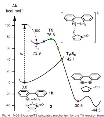
**1b** to the CC bond of **2**. Electronic energies in kcal mol<sup>-1</sup> are given relative to the ground-state reaction complex. The colored points mark the points of the reaction pathway that were investigated in detail in later sections of
