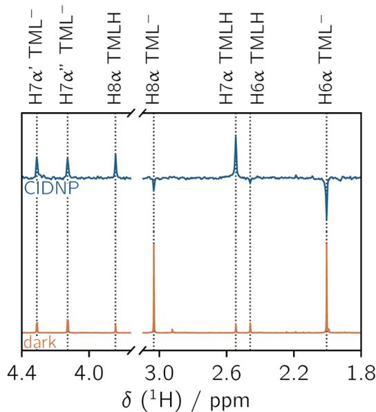
Fig. 3 Dark NMR (orange) and transient photo-CIDNP (blue) spectra of TML (1.6 mM) in a mixture of H<sub>2</sub>O and D<sub>2</sub>O (98.5:1.5, v/v) at pH 12.7. The ratio of TMLH: TML<sup>-</sup> is 1: 7. The dark NMR and photo-CIDNP spectra were measured with 16 and 256 scans, respectively. The sample was irradiated at 425 nm with 4.2 mJ.
