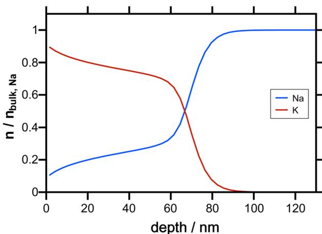
Fig. 1 Concentration depth profile – CAIT benchmark calculation.
