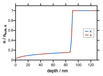
Fig. 4 Concentration depth profile – poling benchmark calculation.
