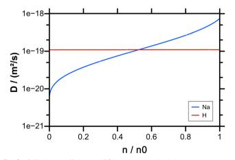
Fig. 8 Diffusion coefficient – APS benchmark calculation.
