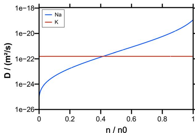
Fig. 2 Diffusion coefficient – CAIT benchmark calculation.
