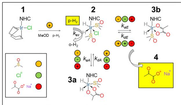
**Scheme 1** Pyruvate hyperpolarization by SABRE. Free pyruvate is obtained as a reversible process *via*  $[\text{Ir}(\text{H})_2(\kappa^2\text{-pyruvate})(\text{DMSO})(\text{NHC})]$  (**3**), whereas hydrogen exchange is mediated by  $[(\text{IrCl}(\text{H})_2(\text{DMSO})_2(\text{NHC}))]$  (**2**) as detailed by Duckett *et al.* in ref. 51.
