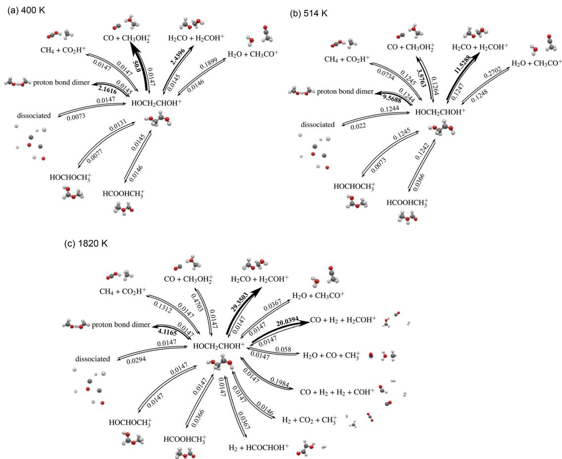
Fig. 4 Reaction rate constants of the reactions involving the protonated glycolaldehyde with other species at (a) 400 K, (b) 514 K, and (c) 1820 K. The unit of the reaction rate constants is  $\text{ps}^{-1}$ .
