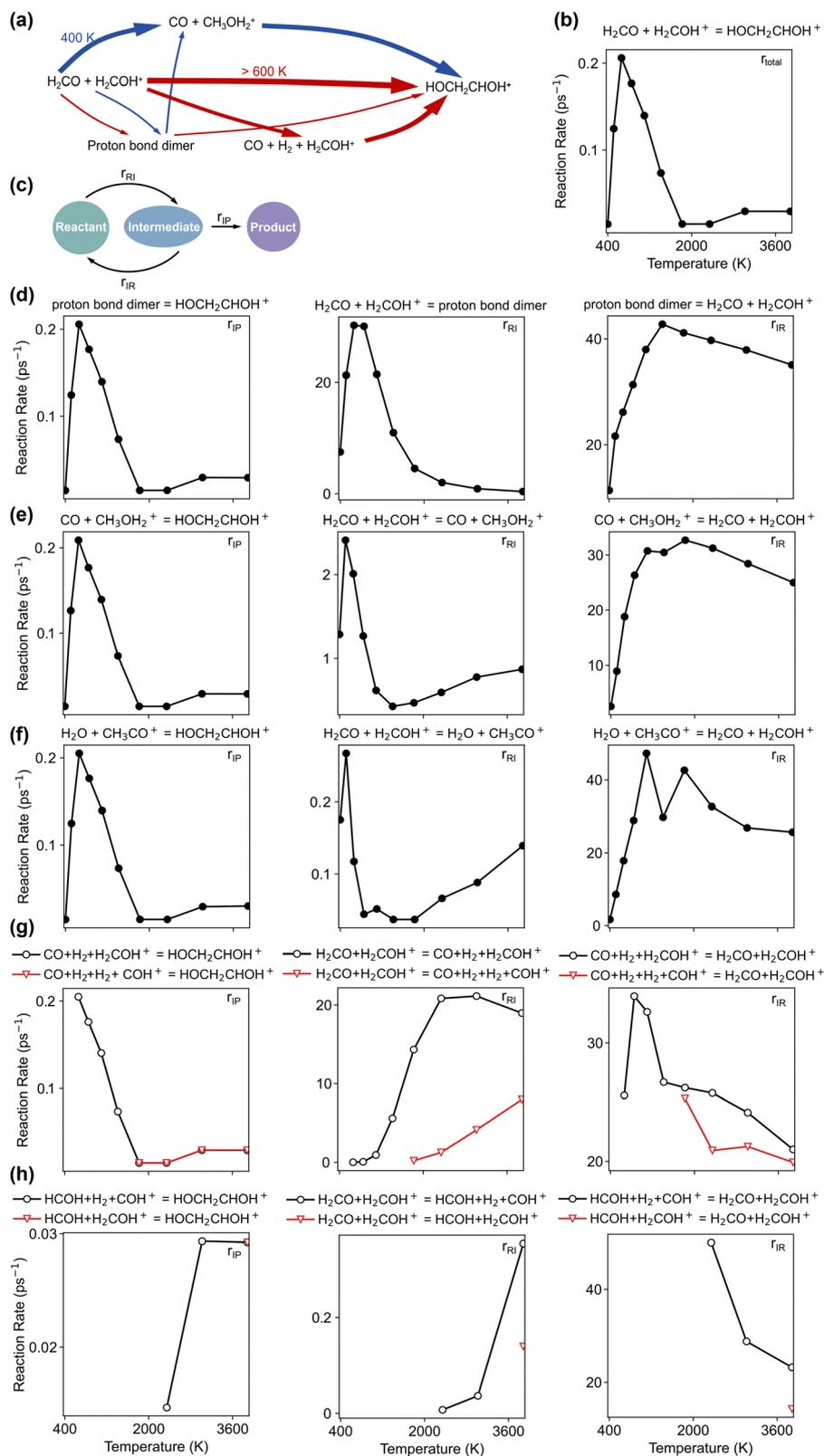
**Fig. 5** Reaction rate constants of the reactions involving the important intermediates. (a) Summary of the reaction pathways at different temperatures. (b) The reaction rate constant of the total reaction as a function of temperature. (c) The reaction rate constants of the reactions involving the important intermediates. (d)–(h) The calculated reaction rate constants  $r_{\text{IP}}$ ,  $r_{\text{RI}}$  and  $r_{\text{IR}}$  as a function of temperature for each reaction.
