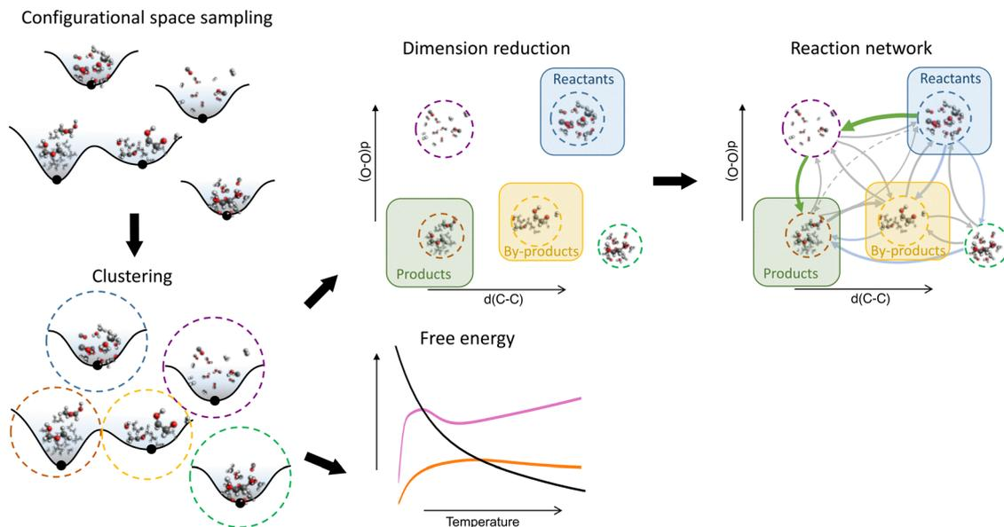
**Fig. 1** Scheme of the methodology employed in this work. AIMD samples the configurational space combined with REMD. Then the sampled configurations are clustered. With the MBAR approach and MSM, the free energy curves are then estimated, and the detailed reaction network about the transitions between different clusters of configurations is constructed.
