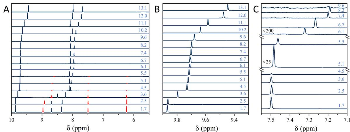
Fig. 2  $^1\text{H-NMR}$  spectra of aqueous 4IC from pH 1 to 13. pH increases from bottom to top, as it is indicated in the right side of each spectra. (A) Shift of aromatic protons (2 and 5) with the aldehyde form in black and diol form in red. (B) Shift of aldehyde proton (6). (C) Shift of nitrogen proton (1).
