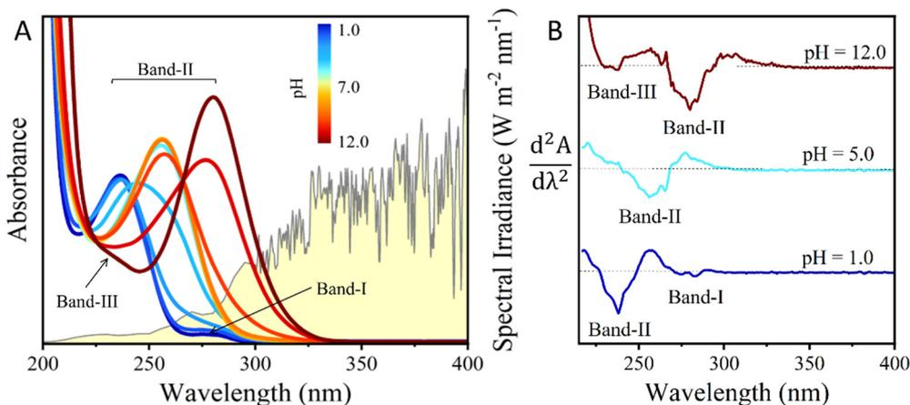
Fig. 1 (A) Absorbance spectra of a solution of 100 mM of 4IC at different pHs – in yellow: solar spectral irradiance (data from NOAA, LASP spectral solar irradiance).<sup>47</sup> (B) 2nd derivative of the spectrum to better identify absorption bands.
