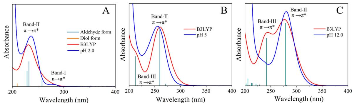
**Fig. 6** Comparison of the theoretical (red line) and experimental (blue line) optical absorption spectra at different pHs. (A) pH 2.0; (B) pH 5.0; (C) pH 12.0. At pH 5.0 and 12.0, only the aldehyde form is used to simulate the spectrum. Level of theory is B3LYP/6-311++G(d,p) (gas phase). While all transitions correspond to mixed  $n \rightarrow \pi^*$  and  $\pi \rightarrow \pi^*$  character, the dominant transition for each band is indicated below the band designation.
