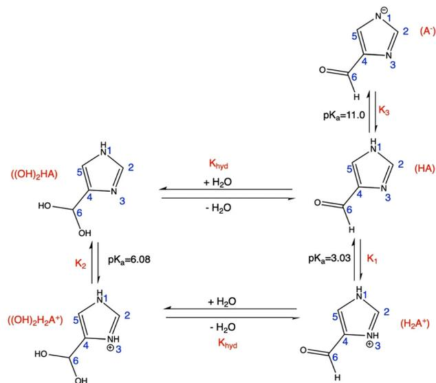
Scheme 1 The associated protonation and hydration equilibrium reactions that occur in aqueous solution for 4IC. Each species is labeled in red in which HA refers to 4-imidazolecarboxaldehyde.
