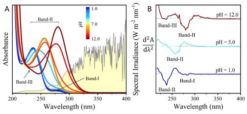
Fig. 1 (A) Absorbance spectra of a solution of 100 mM of 4IC at different pHs – in yellow: solar spectral irradiance (data from NOAA, LASP spectral solar irradiance).<sup>47</sup> (B) 2nd derivative of the spectrum to better identify absorption bands.
