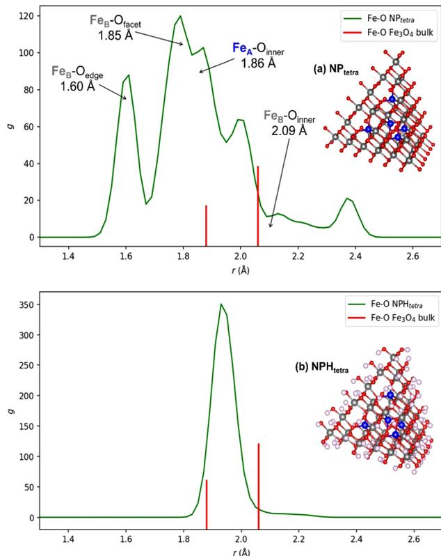
Fig. 7 The partial RDF  $g$  for Fe–O in (a)  $\text{NP}_{\text{tetra}}$  and (b)  $\text{NPH}_{\text{tetra}}$  shown as a green curve. Red vertical markers indicate Fe–O bond distances in magnetite ( $\text{Fe}_3\text{O}_4$ ) bulk for comparison. The numerical values in the RDF spectrum of  $\text{NP}_{\text{tetra}}$  represent average interatomic distances between Fe and O at different coordination sites within the nanoparticle.
