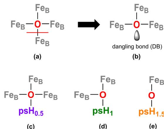
**Fig. 4** Schematic representation of (a) oxygen atom in bulk-like coordination environment and (b) the formation of a dangling bond (DB) upon bond cleavage. Passivation of (c) one DB, (d) two DBs and (e) three DBs using pseudo-hydrogen atoms.
