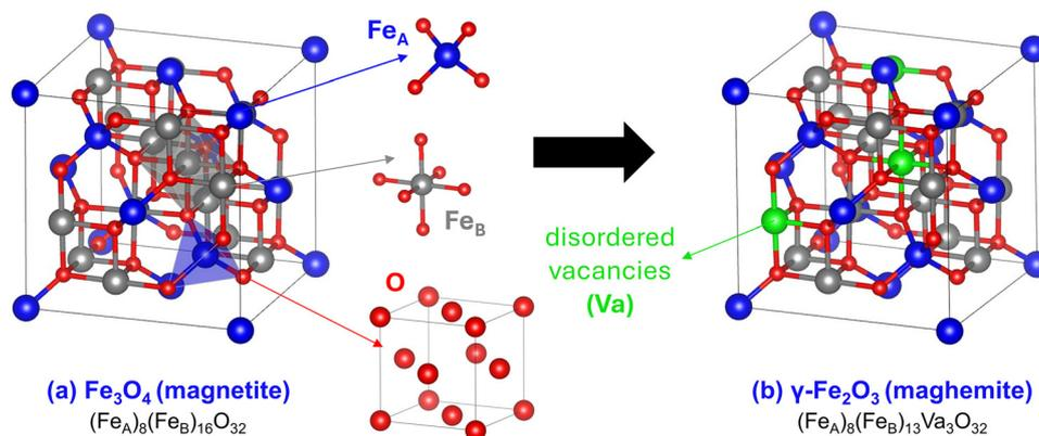
Fig. 2 Inverse spinel structure of (a) magnetite ( $\text{Fe}_3\text{O}_4$ ) and (b) vacancies containing maghemite ( $\gamma\text{-Fe}_2\text{O}_3$ ). Red spheres denote the O atoms in face-centered cubic (fcc) lattice. Blue and grey spheres correspond to the tetrahedral ( $\text{Fe}_A$ ) and octahedral ( $\text{Fe}_B$ ) iron atoms, respectively. Green spheres correspond to vacancies Va.
