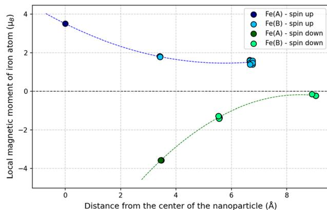
**Fig. 10** Dependence of the magnitude of the magnetic moment on the distance of tetrahedral Fe<sub>A</sub> and octahedral Fe<sub>B</sub> iron atoms from the center of NP<sub>tetra</sub>. The dashed lines are included merely to guide the eye and do not represent interpolated data.
