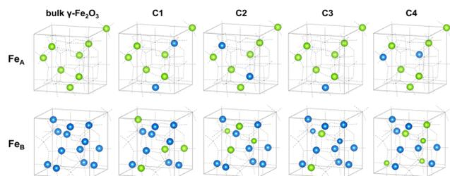
Fig. 12 The magnetic arrangement of C1–C4 configurations, showing only iron atoms. The grey dashed lines represent Fe–O bonds. Green and blue spheres indicate spin-down ( $\downarrow$ ) and spin-up ( $\uparrow$ ) orientation of the atomic magnetic moment, respectively. The size of each iron sphere is directly proportional to the absolute value of its magnetic moment.
