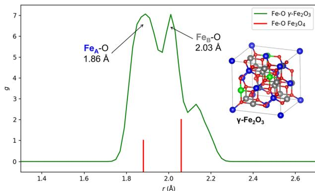
Fig. 6 The partial RDF  $g$  for Fe–O in maghemite ( $\gamma$ - $\text{Fe}_2\text{O}_3$ ) depicted as a green curve. Red vertical markers indicate Fe–O bond distances in magnetite ( $\text{Fe}_3\text{O}_4$ ) for comparison. The function  $g$  represents the probability density of finding a particle at the distance  $r$  from a reference particle.
