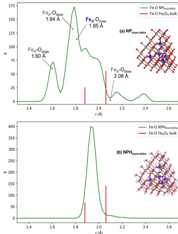
Fig. 8 The partial RDF  $g$  for Fe–O in (a)  $\text{NP}_{\text{trunc-tetra}}$  and (b)  $\text{NPH}_{\text{trunc-tetra}}$  shown as a green curve. Red vertical markers indicate Fe–O bond distances in magnetite ( $\text{Fe}_3\text{O}_4$ ) bulk for comparison. The numerical values in the RDF spectrum of  $\text{NP}_{\text{trunc-tetra}}$  represent average interatomic distances between Fe and O at different coordination sites within the nanoparticle.
