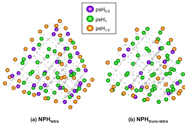
Fig. 5 Distribution of pseudo-hydrogen atoms across (a)  $\text{NPH}_{\text{tetra}}$  and (b)  $\text{NPH}_{\text{trunc-tetra}}$ . The different colors represent assigned effective charges:  $\text{psH}_{0.5}$  (purple spheres),  $\text{psH}_1$  (green spheres) and  $\text{psH}_{1.5}$  (orange spheres).
