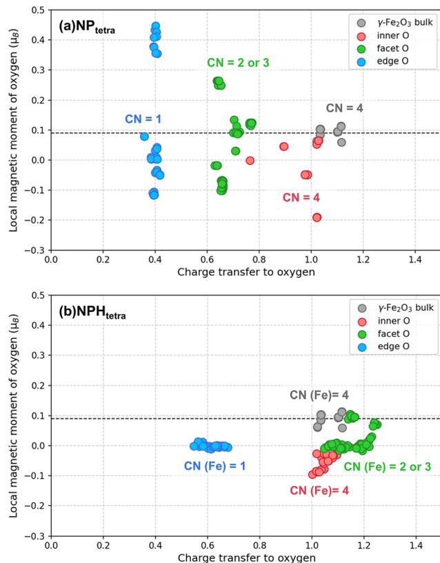
Fig. 14 Dependence of the local magnetic moment of oxygen on charge transfer to oxygen from iron atoms in (a)  $\text{NP}_{\text{tetra}}$  and from both iron and psH atoms in (b)  $\text{NPH}_{\text{tetra}}$ . Oxygen atoms located on the inside ( $\text{O}_{\text{inner}}$ ), on the facets ( $\text{O}_{\text{facet}}$ ) and at the edges ( $\text{O}_{\text{edge}}$ ) of the NP models are color-coded accordingly.
