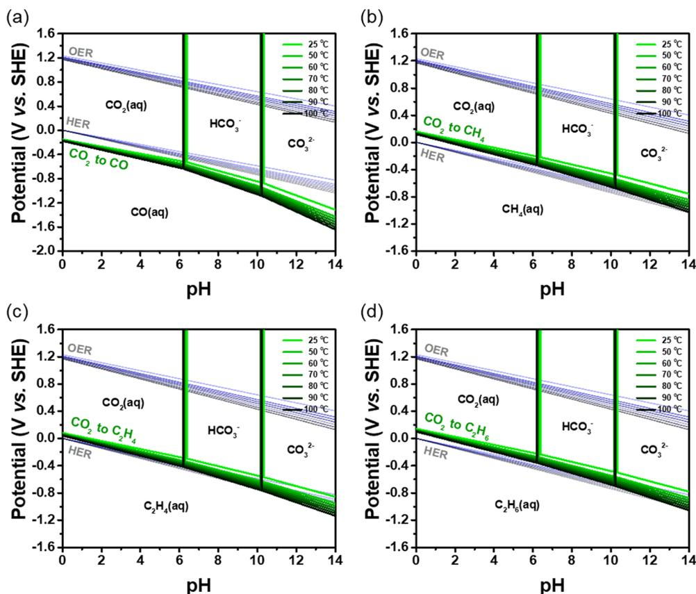
Fig. 1 Pourbaix diagrams of hydrocarbons including (a) CO, (b) CH<sub>4</sub>, (c) C<sub>2</sub>H<sub>4</sub>, and (d) C<sub>2</sub>H<sub>6</sub> using CO<sub>2</sub>(aq) as a function of temperature from 25 to 100 °C.
