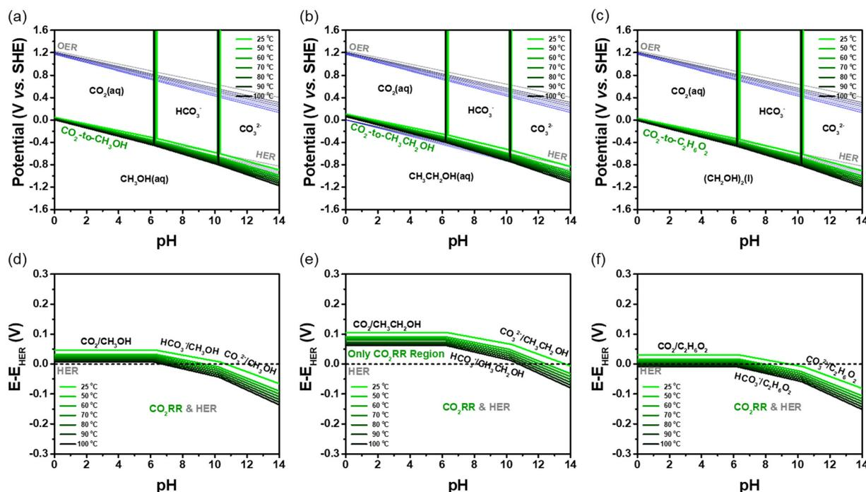
Fig. 6 Pourbaix diagrams of (a) methanol, (b) ethanol, and (c) ethylene glycol as a function of temperature from 25 to 100 °C. The potential gap between CO<sub>2</sub>RR and HER for the formation of (d) CH<sub>3</sub>OH, (e) CH<sub>3</sub>CH<sub>2</sub>OH, and (f) C<sub>2</sub>H<sub>6</sub>O<sub>2</sub> as a function of temperature (25–100 °C).
