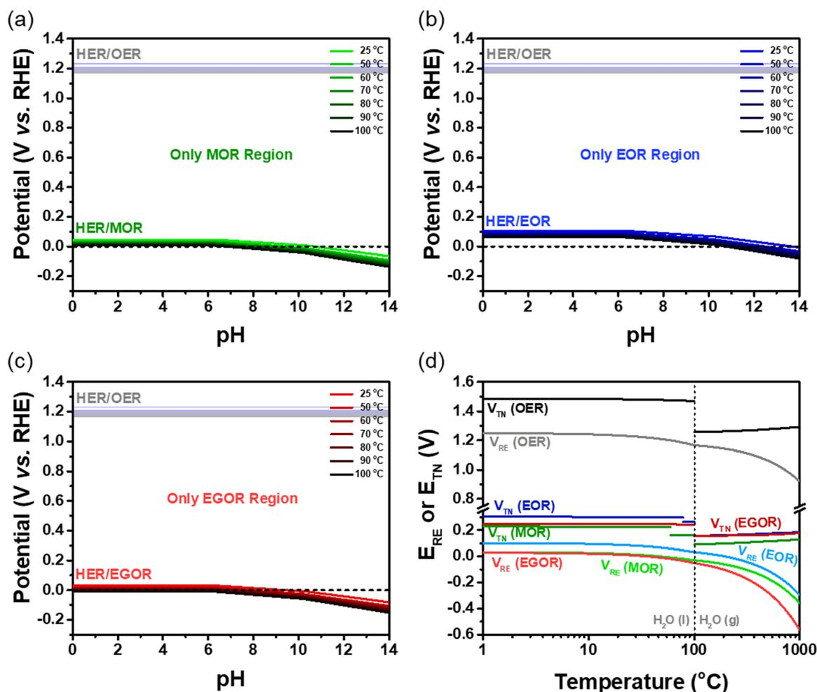
Fig. 8 Potential difference between water electrolysis and assisted water electrolysis using (a) methanol, (b) ethanol, and (c) ethylene glycol as a function of temperature from 25 to 100 °C. (d)  $V_{RE}$  and  $V_{TN}$  of water electrolysis and assisted water electrolysis using alcohols as a function of temperature from 0 to 1000 °C.
