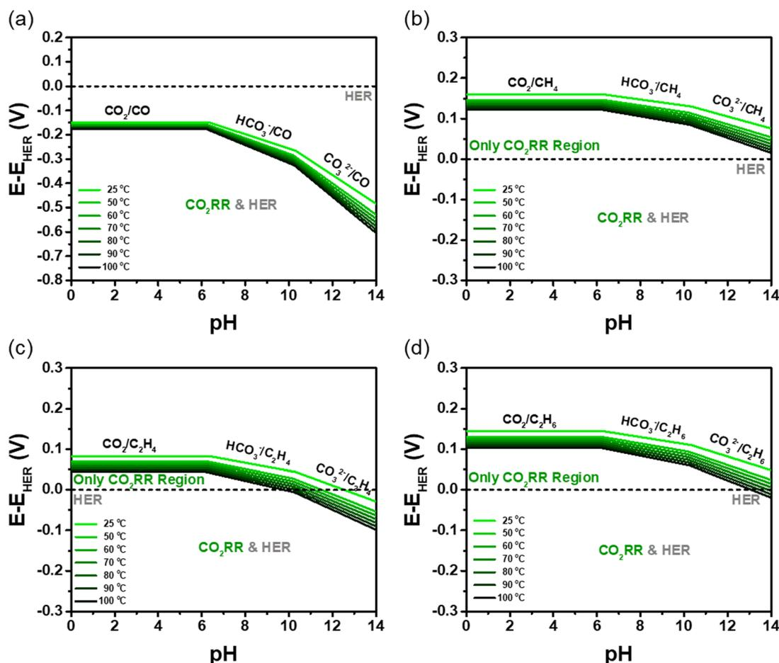
Fig. 2 Potential gap between CO<sub>2</sub>RR and HER for the formation of (a) CO, (b) CH<sub>4</sub>, (c) C<sub>2</sub>H<sub>4</sub>, and (d) C<sub>2</sub>H<sub>6</sub> as a function of temperature (25–100 °C).
