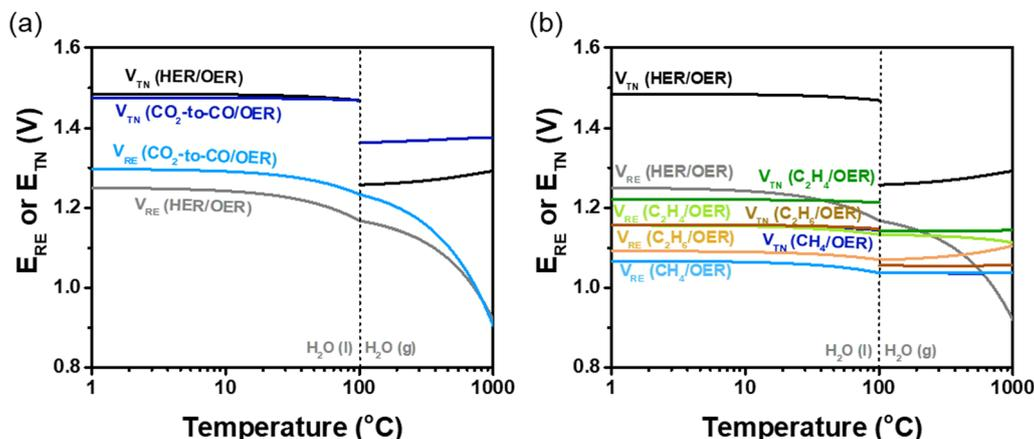
Fig. 3 Theoretical potentials ( $V_{TN}$  and  $V_{RE}$ ) of (a) CO<sub>2</sub>RR to CO and (b) hydrocarbons, as a function of temperature from 0 to 1000 °C.
