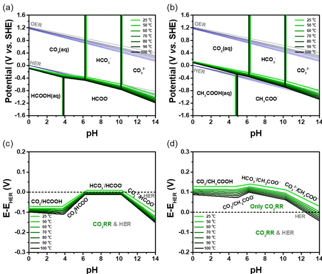
Fig. 4 Pourbaix diagrams of organic acids, including (a) formic acid and (b) acetic acid, using CO<sub>2</sub>(aq) as a function of temperature from 25 to 100 °C. Potential gap between CO<sub>2</sub>RR and HER for the formation of (c) HCOOH and (d) CH<sub>3</sub>COOH as a function of temperature (25–100 °C).
