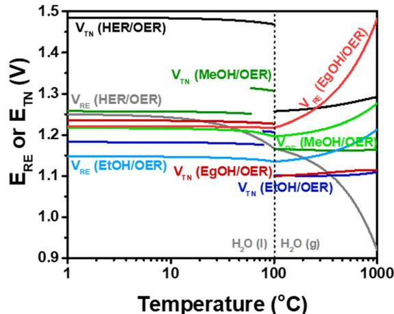
Fig. 7 Theoretical potentials ( $V_{\text{TN}}$  and  $V_{\text{RE}}$ ) of CO<sub>2</sub>-to-alcohol reactions as a function of temperature from 0 to 1000 °C.
