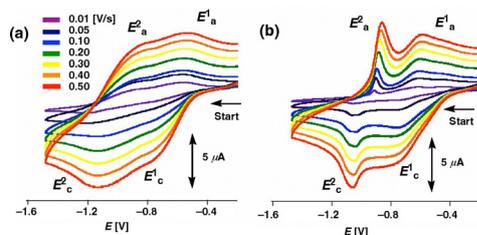
Fig. 2 Solid-state CV images of **1** in MeCN solutions of (a) <sup>n</sup>Pen<sub>4</sub>NBr and (b) <sup>n</sup>Oct<sub>4</sub>NBr electrolyte salts. The velocity was changed from 0.01 to 0.5 V s<sup>-1</sup> (vs. Ag/Ag<sup>+</sup>, WE: glassy carbon, RE: Pt wire).
