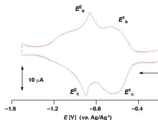
Fig. 4 Semi-differential solid-state CV curve of **1** measured in MeCN solution with the  $\text{Ph}_4\text{PBr}$  electrolyte salt.
