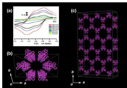
**Fig. 1** (a) Solid-state CV of the single crystals of **1** in MeCN with  $t\text{Bu}_4\text{NPF}_6$  as the electrolyte salt. The velocities were changed from 10 to 500  $\text{mV s}^{-1}$ . (b) Down view along the  $c$  axis showing the 1-D nanochannel unit. (c) View parallel to the  $ab$  plane showing the 2-D honeycomb sheet structure formed by H-bonds between the  $[\text{Ru}^{\text{III}}(\text{Hbim})_3]$  of **1**.
