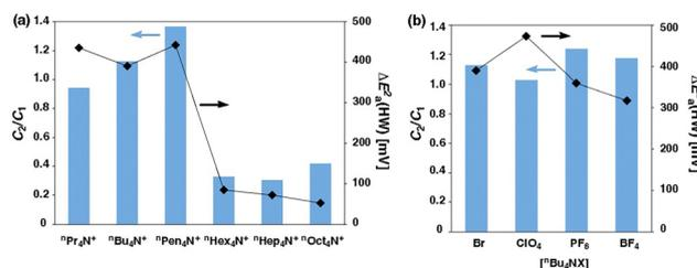
Fig. 3 Ratios of the current areas of the primary reduction peaks  $E_c^1$  ( $C_1$ ) to those of the secondary oxidation peaks  $E_a^2$  ( $C_2$ ) of the solid-state CV curves as bar graphs and the corresponding half-width potentials  $\Delta E_a^2(\text{HW})$  as line graphs of (a) **1** in six electrolyte salts with R<sub>4</sub>N<sup>+</sup> cations of different EIRs and (b) **1** in four electrolyte salts with different X<sup>-</sup> anions of <sup>n</sup>Bu<sub>4</sub>N<sup>+</sup>.
