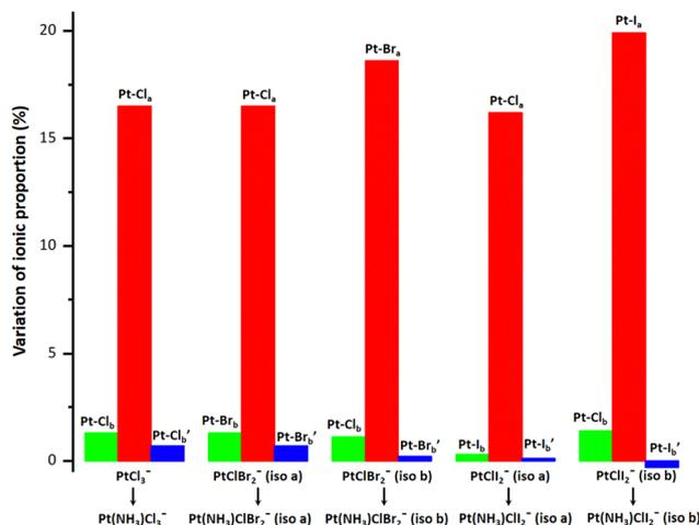
Fig. 4 The difference in ionic proportion of the corresponding Pt–halogen bonds in  $\text{PtClX}_2^-$  and  $\text{Pt}(\text{NH}_3)\text{ClX}_2^-$  ( $X = \text{Cl}, \text{Br}, \text{I}$ ). The calculations were performed at the B3LYP-D3(BJ)/aug-cc-pVTZ-(pp) level of theory.
