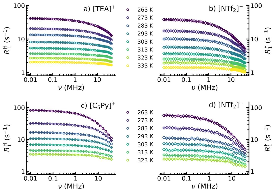
Fig. 2 Temperature dependent NMRD profiles for  $^1\text{H}$  (a) and (c) plotted as circles and  $^{19}\text{F}$  (b) and (d) plotted as diamonds in the ionic liquids [TEA][NTf<sub>2</sub>] (a) and (b) and [C<sub>5</sub>Py][NTf<sub>2</sub>] (c) and (d). The solid lines correspond to the model fits according to eqn (1), (5), (9) and (12) for [TEA][NTf<sub>2</sub>] as well as to eqn (1), (6), (9) and (12) for [C<sub>5</sub>Py][NTf<sub>2</sub>].
