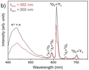
Fig. 5 Emission spectra of compounds **8** (a) and **5** (b) at the indicated  $\lambda_{\rm exc}$ in solid state at room temperature
