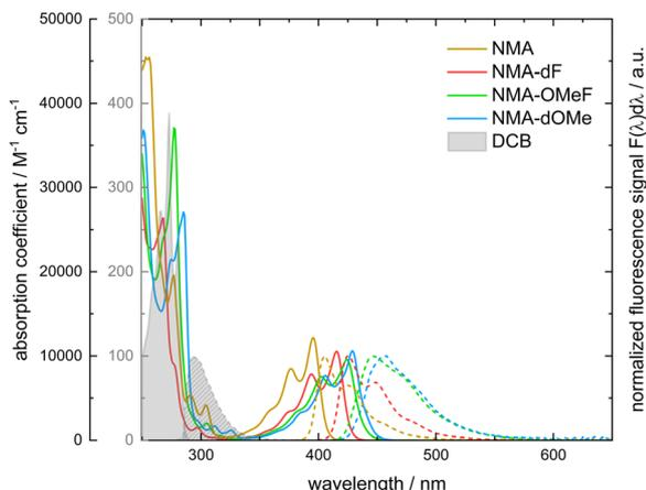
**Fig. 3** Absorption coefficient (solid lines) and fluorescence (normalized, dashed lines) spectra of NMA (yellow), NMA-dF (red), NMA-OMeF (green), NMA-dOMe (blue) and DCB (grey areas) in THF. The black y-axis on the left refers to absorption coefficients of the NMAs, the gray one to absorption coefficients of DCB. For the acquisition of the fluorescence spectra the excitation was tuned to the absorption maxima lowest in energy.
