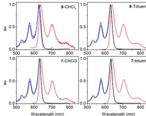
Fig. 1 Absorption, emission and excitation spectra of dyes **7** and **8** in CHCl<sub>3</sub> (left panels) and toluene (right panels). Spectra recorded in CCl<sub>4</sub>, THF, CH<sub>2</sub>Cl<sub>2</sub> and benzonitrile are included in the ESI.†
