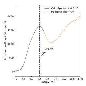
Fig. 5 In blue, a calculated absorption spectrum of water at 0  $^{\circ}\text{C}$  is presented using extrapolated fitting parameters from the work of Marin et al.<sup>6</sup> The calculated spectrum matches the measured spectrum of a sheet thickness of 41 nm after background subtraction and normalization.
