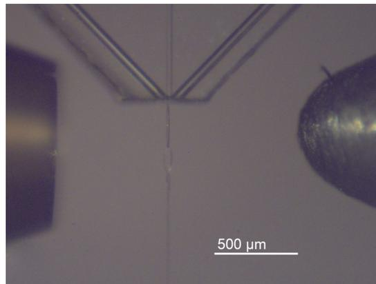
Fig. 2 Close-up of the interaction region. The entrance skimmer towards the gas filter is seen on the left. On the right is the detector skimmer acting as an exit slit, defining the probe area as well as shielding the photodiode from contamination. The Micronit glass chip with the three channels and the produced liquid sheet can be seen in between.
