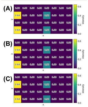
Fig. 3 SAED patterns for a  $2^3 \times 2^2$  shaped one layered CeO<sub>2</sub>(100) surface derived from (A) discrete FT, (B) FFT and (C) QFT. The values are intensities in the heat map
