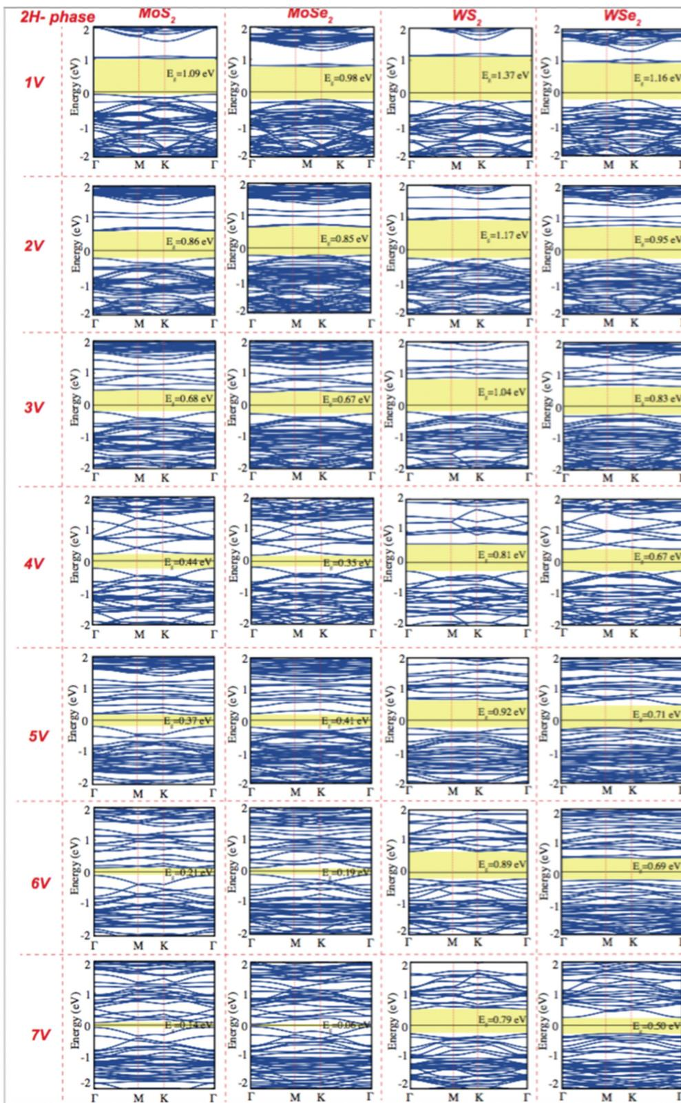
Fig. 4 Electronic band structure of pristine single layer 2H phase MoS<sub>2</sub>, MoSe<sub>2</sub>, WS<sub>2</sub>, and WSe<sub>2</sub> as a function of the concentration of chalcogen vacancy. The black line indicates the Fermi level at zero eV.
