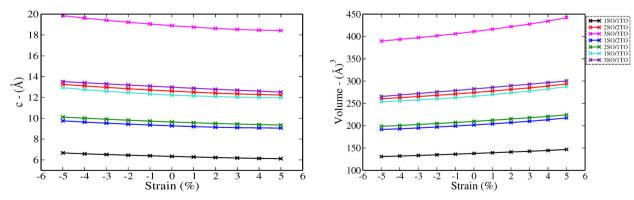
Fig. 3 Structure parameters of nSO/mTO superlattices under biaxial strains from -5% to 5%: c parameters (left) and volumes (right).
