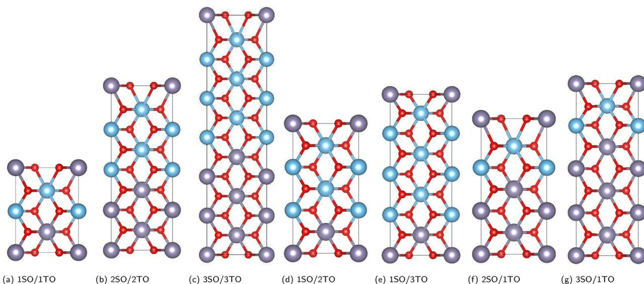
Fig. 1 (a)–(g) Schematic view of  $(\text{SnO}_2)_n/(\text{TiO}_2)_m$  ( $n, m = 1, 2, 3$ ) superlattices, where  $n$  and  $m$  are the number of unit cells of  $\text{SnO}_2$  (SO) and  $\text{TiO}_2$  (TO), respectively (gray, blue, and red colors represent Sn, Ti, and O atoms).
