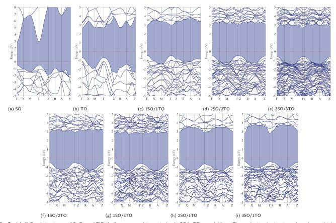
Fig. 8 (a)–(i) Band structures of SnO<sub>2</sub> and TiO<sub>2</sub> bulks compared to unstrained nSO/mTO superlattices. These electronic structures have been obtained at DFT-HSE06 level of theory. The Fermi level is located at zero electron-volt (the blue shaded areas correspond to energies between the highest valence bands and the lowest conduction bands).
