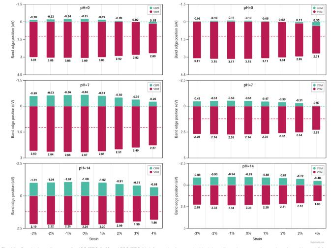
Fig. 14 Band edges alignment for 1SO/3TO (left) and 3SO/3TO (right) superlattices under biaxial tensile and compressive strains when pH equal 0 (upper part), 7 (middle part) and 14 (bottom part). The horizontal dashed lines are the water redox potentials
