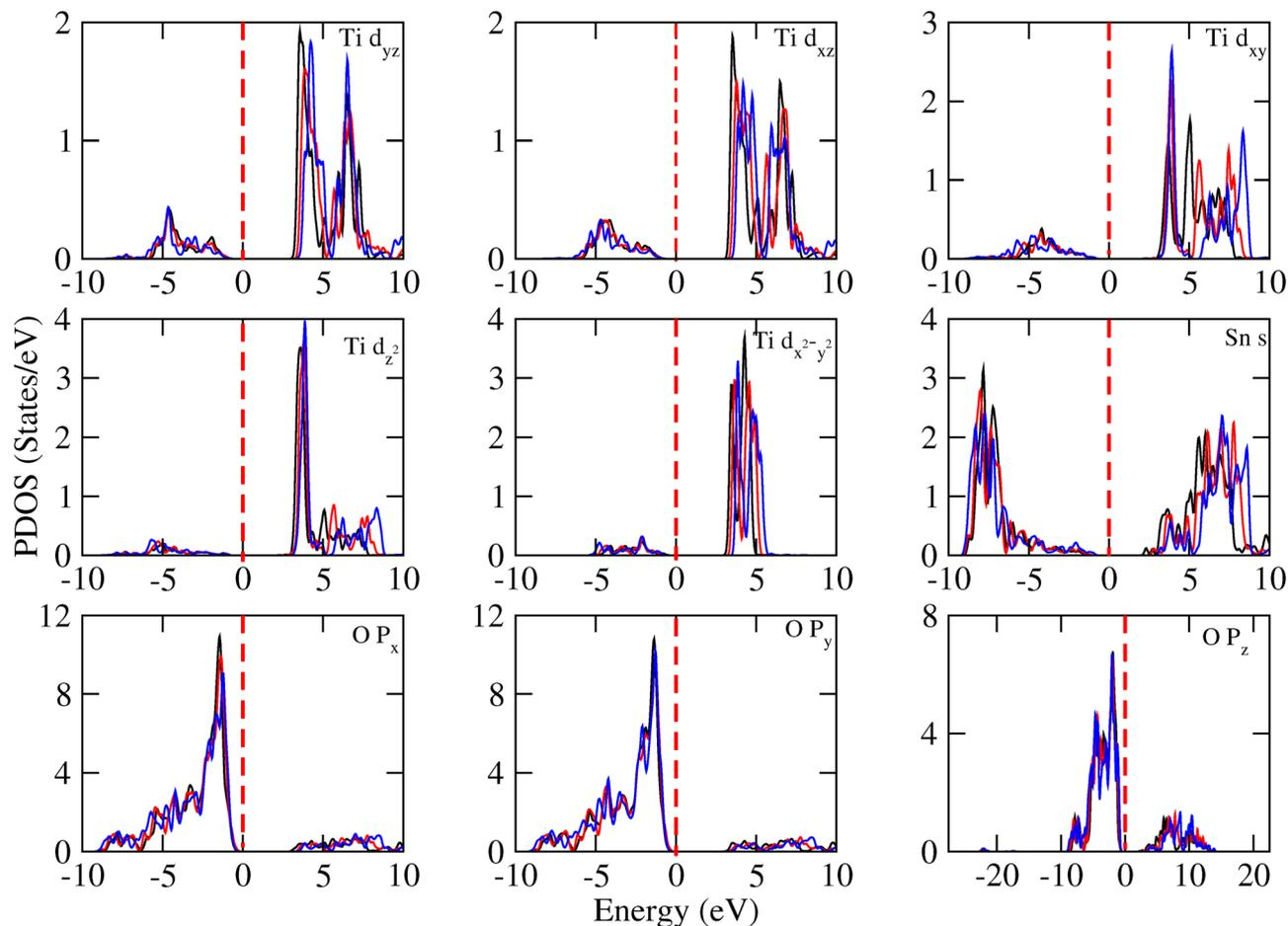
Fig. 12 Contributions into DOS of Ti-d, Sn-s and O-p orbitals for the 3SO/1TO superlattice under upper limits  $-5\%$  (black),  $0\%$  (red) and  $5\%$  (blue) biaxial strains.
