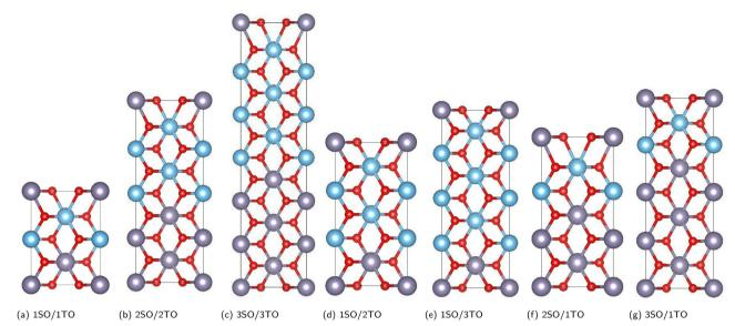
Fig. 1 (a)–(g) Schematic view of  $(SnO_2)_{(n)}/(TiO_2)_{(m)}$  (n,m=1,2,3) superlattices, where n and m are the number of unit cells of  $SnO_2$  (SO) and  $TiO_2$  (TO), respectively (gray, blue, and red colors represent Sn, Ti, and O atoms).
