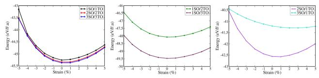
Fig. 4 The total energy-biaxial strain relationship of nSO/mTO superlattices for different stacking periodicity: (n = m) left, (1, m) middle, and (n, 1) right.
