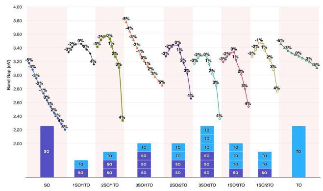
Fig. 10 Biaxial strain effect on the band gap of  $XO_2$  (X = Sn, Ti) metal oxides and nSO/mTO superlattices
