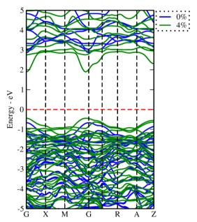
Fig. 11 Band structures for the 2SO/1TO under 0% (blue) and 4% (green) tensile strain. The Fermi level is located at 0 electron-volt
