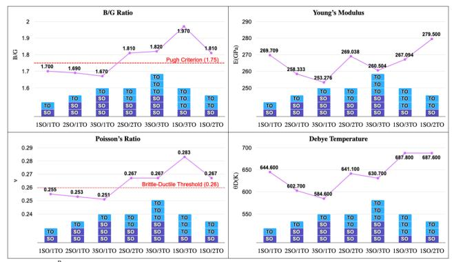
Fig. 6 Evolution of  $\frac{B}{G}$  ratio, Young's modulus (E), Poisson's ratio (n), and Debye temperature ( $\theta_D$ ) of unstrained nSO/mTO superlattices for different (n/m) stacking periodicities.
