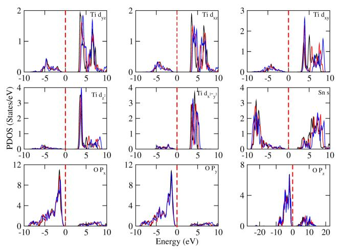
Contributions into DOS of Ti-d, Sn-s and O-p orbitals for the 3SO/1TO superlattice under upper limits -5% (black), 0% (red) and 5% (blue) biaxial Fig. 12 strains
