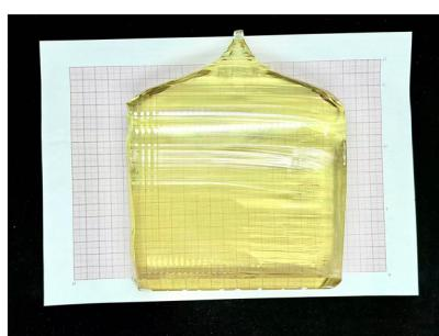
**Growth and characterization of 6 inch  $Ca_3Ta(Ga_{0.25}Al_{0.75})_3Si_2O_{14}$  for high-temperature piezoelectric applications**
