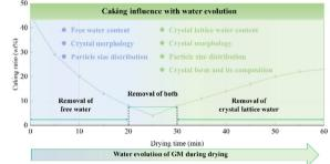
Revealing the relationship between the anti-caking function of wet hydrate crystals and water migration: a case study of glucose monohydrate
