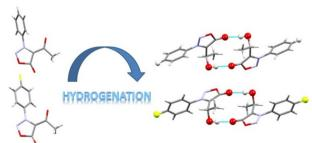
H/F replacement in secondary alcohols of sydnones as examples of isostructural OH···O=C hydrogen bonded dimer structures
