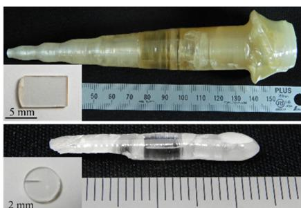
**High-density Nb:YTaO<sub>4</sub> single crystals for X-ray scintillation**
