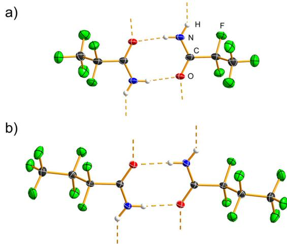
**Fig. 1** R<sub>2</sub><sup>2</sup>(8) hydrogen-bonding motifs in the crystal structures of (a) C<sub>2</sub>F<sub>5</sub>CONH<sub>2</sub> and (b) C<sub>3</sub>F<sub>7</sub>CONH<sub>2</sub>. Hydrogen bonds are shown as dashed orange lines. Displacement ellipsoids are drawn at the 50% probability level, and hydrogen atoms are represented as spheres of arbitrary radius.
