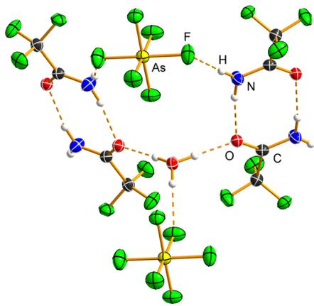
**Fig. 5**  $\text{R}_6^6(14)$  hydrogen-bonded cluster in the crystal structure of the  $\text{H}_3\text{O}[\text{AsF}_6]\cdot 2\text{CF}_3\text{CONH}_2$  salt cocrystal. Hydrogen bonds are shown by dashed orange lines. Displacement ellipsoids are drawn at the 50% probability level, and hydrogen atoms are represented as spheres of arbitrary radius.
