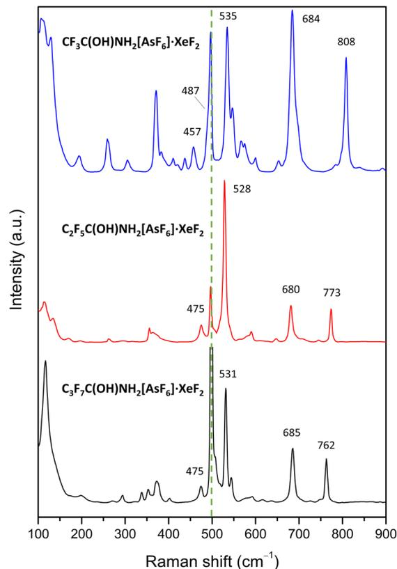
Fig. 8 Raman spectra of  $XeF_2$  salt cococrystals with protonated amides recorded at low temperatures ( $-90\text{ }^\circ\text{C}$ ). The green dashed line is placed at the position of free  $XeF_2$  ( $497\text{ }cm^{-1}$ )<sup>41</sup> which was observed as an impurity in the reactions.
