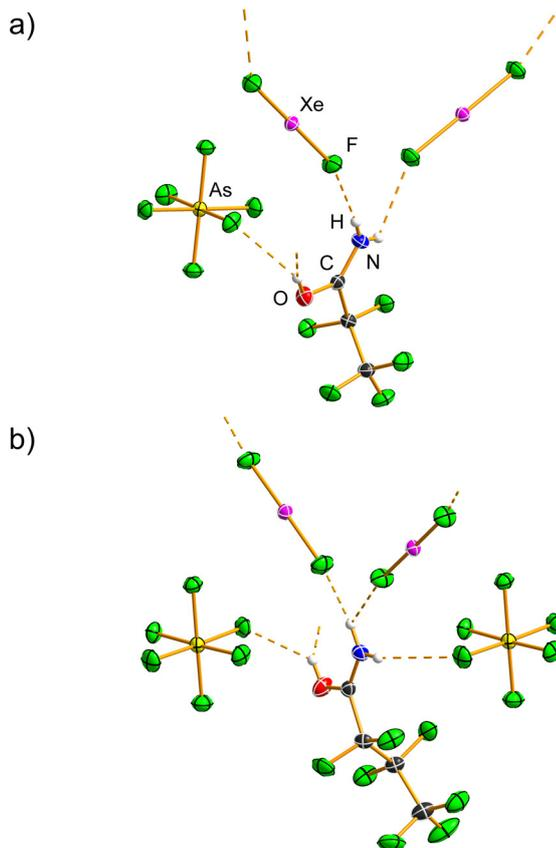
Fig. 7 Hydrogen bonds (dashed orange lines) in the crystal structures of the salt cococrystals (a)  $C_2F_5C(OH)NH_2[AsF_6] \cdot XeF_2$  and (b)  $C_3F_7C(OH)NH_2[AsF_6] \cdot XeF_2$ . The OH groups are bifurcated hydrogen-bond donors; however, two  $[AsF_6]^-$  anions have been omitted for clarity. Displacement ellipsoids are drawn at the 50% probability level, and hydrogen atoms are represented as spheres of arbitrary radius.
