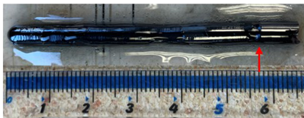
Fig. 4 The \text{Ca}_2\text{Fe}_2\text{O}_5 crystal mounted in resin in preparation of cutting with a diamond wire saw. The scale bar is in centimetres. The red arrow marks the seeding point.
