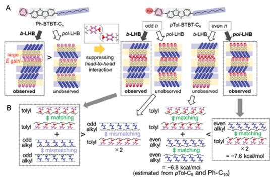
Fig. 9 Schematics of the layer-by-layer stacking combinations. A) Schematics of Ph-BTBT-Cn (left) and pTol-BTBT-Cn (right). The orange and blue areas show BTBT-core layers and alkyl chain layers, respectively. B) Schematics of the affinities in the layer surface for tolyl groups, odd-n alkyl chains, and even-n alkyl chains. The black dashed lines schematically show the boundary of the space-filling surface. Reprinted with permission from ref. 83. Copyright 2024, WILEY.
