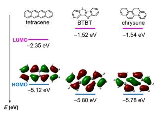
**Fig. 1** Calculated energy levels and HOMOs (density functional theory (DFT) calculations, B3LYP/6-311q(d,p) level).
