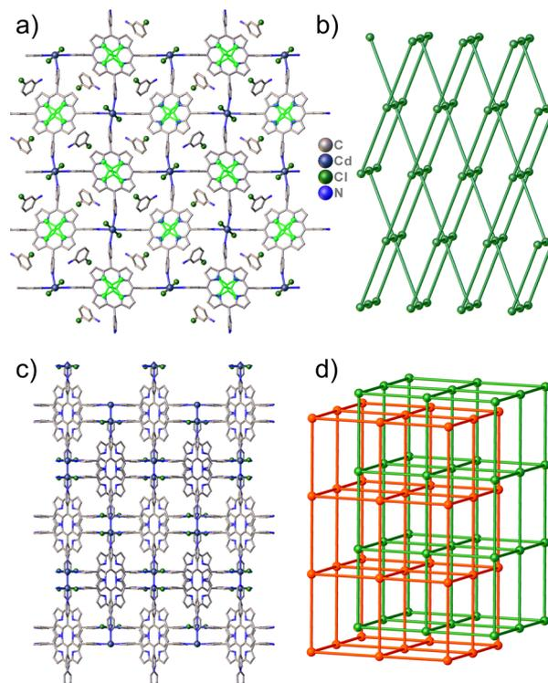
**Fig. 1** Crystal structures ([100] view) and topological representations for UB-MOF-1 (a and b) and ESRF-MOF-1 (c and d), respectively. Hydrogens are omitted and TCE molecules sitting atop the porphyrin rings are depicted in bright green for clarity.
