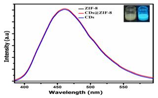
Fig. 4 Fluorescence emission spectra of CDs, ZIF-8, and CDs@ZIF-8. Images of CDs@ZIF-8 dispersed in ethanol under visible light (left) and 365 nm UV illumination (right).
