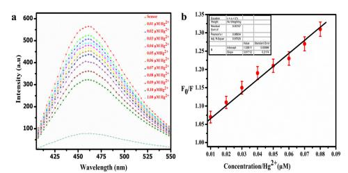
Fig. 8 (a) Fluorescence emission spectra of CDs@ZIF-8 with varying concentrations of  $Hg^{2+}$  ions. (b) Linear correlation between the relative fluorescence intensity ( $F_0/F$ ) and  $Hg^{2+}$  concentration ranging from 0.01 to 1.00  $\mu$ M, demonstrating quantitative sensing capability.
