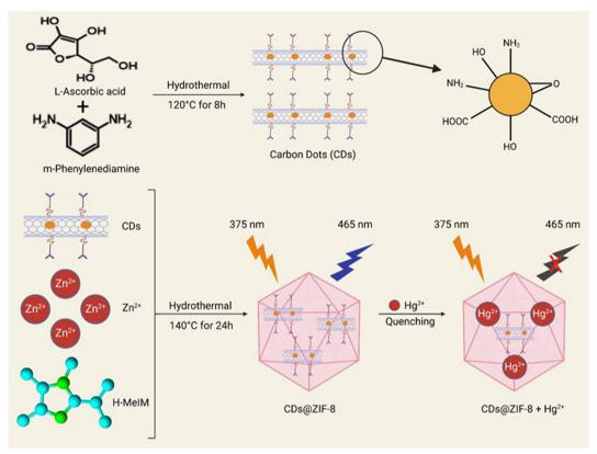
Scheme 1 Schematic representation of the preparation of luminescent CDs@ZIF-8 hybrid nano-sensor and its application as a fluorescent sensor for  $Hg^{2+}$  detection.
