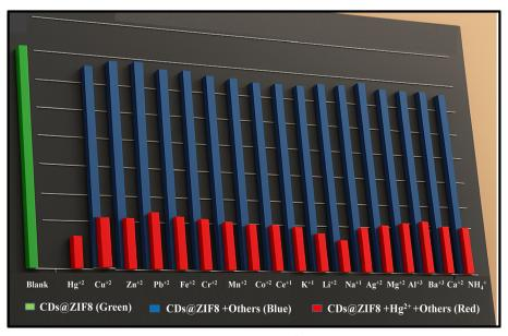
Fig. 7 Evaluation of the anti-interference capability of CDs@ZIF-8 toward Hg<sup>2+</sup> detection in the presence of various competing metal ions, highlighting its high selectivity and stability.
