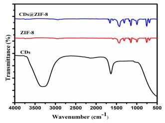
Fig. 2 FT-IR spectra of CDs, ZIF-8, and CDs@ZIF-8.
