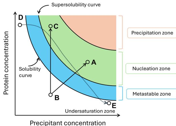
Fig. 1 Protein phase diagram reporting various possible pathways to achieve supersaturation according to batch (A), vapor diffusion (B to A), dialysis (B to C), and counter-diffusion (D to E) crystallization.
