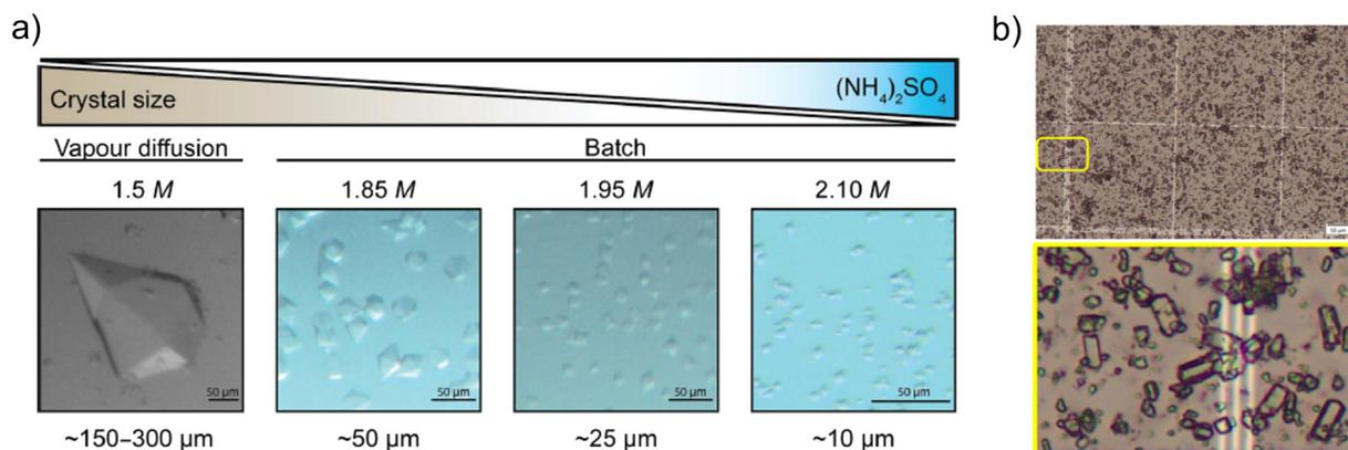
Fig. 8 (a) Crystal size of *E. coli* l-aspartate  $\alpha$ -decarboxylase as a function of ammonium sulfate concentration. Reprinted with permission.<sup>129</sup> Copyright 2020, International Union of Crystallography. (b) HEWL microcrystals obtained with lanthanide complexes (TbXo4 crystallophore). Reprinted with permission.<sup>131</sup> Copyright 2024, American Chemical Society.
