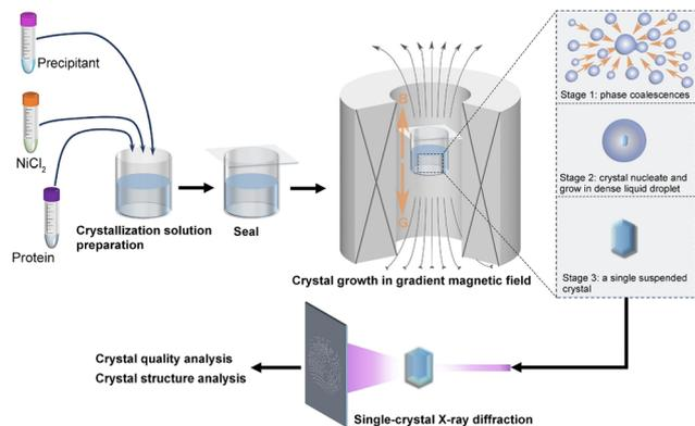
Fig. 7 Schematics of the set-up of contactless crystallization. Reprinted with permission.<sup>113</sup> Copyright 2024, Elsevier Science.
