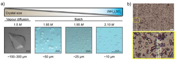
Fig. 8 (a) Crystal size of *E. coli* l-aspartate  $\alpha$ -decarboxylase as a function of ammonium sulfate concentration. Reprinted with permission. (b) HEWL microcrystals obtained with lanthanide complexes (TbXo4 crystallophore). Reprinted with permission. (131 Copyright 2024, American Chemical Society.
