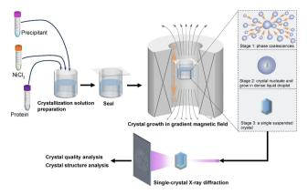
Fig. 7 Schematics of the set-up of contactless crystallization. Reprinted with permission. 113 Copyright 2024, Elsevier Science.
