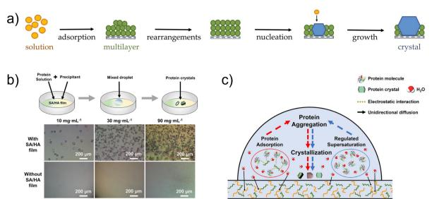
Fig. 3 (a) Schematics of an adsorption-mediated protein crystallization process. Reprinted with permission.<sup>58</sup> Copyright 2024, Elsevier Science. (b) Film-assisted protein crystallization: schematics and optical microscope images of HEWL crystallization with and without films. (c) Mechanism for film-assisted protein crystallization. Reprinted with permission. <sup>59</sup> Copyright 2025, Elsevier Science.
