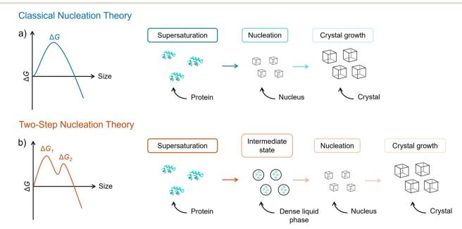
Fig. 2 Comparison between the evolution of the total free energy vs. size and the mechanisms of nucleation proposed by (a) Classical Nucleation Theory and (b) Two-step Nucleation Theory.
