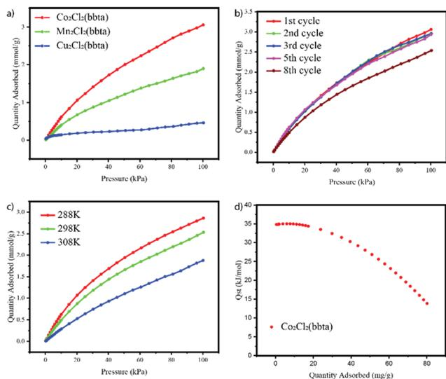
**Fig. 3** The single-component CO adsorption isotherms of (a)  $\text{M}_2\text{Cl}_2(\text{bbta})$  ( $\text{M} = \text{Co}, \text{Mn}, \text{Cu}$ ) at 298 K; (b)  $\text{Co}_2\text{Cl}_2(\text{bbta})$  after multiple cycles; (c)  $\text{Co}_2\text{Cl}_2(\text{bbta})$  at 288 K, 298 K and 308 K. (d) The isosteric heats ( $Q_{\text{st}}$ ) of CO adsorption of  $\text{Co}_2\text{Cl}_2(\text{bbta})$  calculated from isotherms collected at 288 K, 298 K and 308 K.
