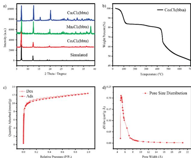
Fig. 2 (a) PXRD patterns of  $\text{M}_2\text{Cl}_2(\text{bbta})$ . (b) The TGA plots of  $\text{Co}_2\text{Cl}_2(\text{bbta})$ . (c)  $\text{CO}_2$  adsorption–desorption isotherms of  $\text{Co}_2\text{Cl}_2(\text{bbta})$  at 195 K, and (d) pore size distribution (H–K function) of  $\text{Co}_2\text{Cl}_2(\text{bbta})$ .
