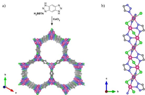
Fig. 1 (a) Crystal structure of  $\text{Co}_2\text{Cl}_2(\text{bbta})$  viewed along the *c*-axis. (b) Structure of a helical cobalt-chloride-triazolate chain running along the *c*-axis (Co, pink; Cl, green; N, blue; C, grey; H, white).
