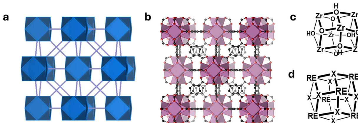
Fig. 1 (a) **fcu** net, (b) structure of UiO-66, (c)  $[\text{Zr}_6\text{O}_4\text{OH}_4]^{12+}$  cluster of Zr-UiO-66, and (d)  $[\text{RE}_6\text{X}_8]^{10+}$  cluster of RE-UiO-66, where X = OH or F.
