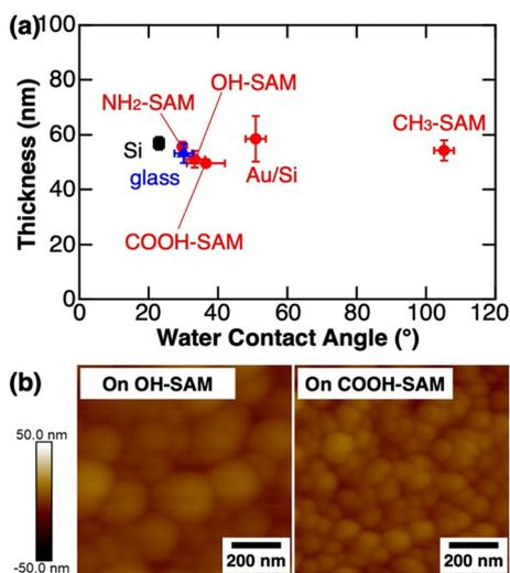
**Fig. 7** (a) Thickness of ZIF-8 films formed on different substrates using a Pt electrode (6 mm in diameter) in a methanol solution containing 10 mM  $\text{ZnCl}_2$  and 20 mM Hmim at  $E = -1 \text{ V}$  with  $h = 50\text{--}150 \text{ }\mu\text{m}$  for  $t = 15 \text{ min}$ .<sup>34</sup> (b) AFM images of ZIF-8 films formed on an OH-SAM and a COOH-SAM.<sup>34</sup> Adapted with permission from ref. 34. Copyright 2025 IOP Publishing Limited on behalf of the Electrochemical Society.
