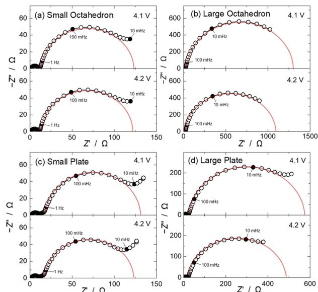
**Fig. 2** Nyquist plots of Li/NCM cells measured at 4.1 and 4.2 V. The diluted NCM electrodes contained 10 wt% NCM. Morphologies of NCM: (a) small octahedral, (b) large octahedral, (c) small plate-like, and (d) large plate-like particles.
