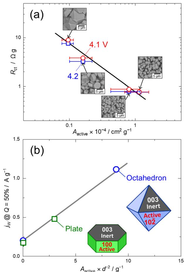
**Fig. 4** (a) Plots of  $R_{ct}$  versus  $A_{active}$  in double-logarithmic scales. Red and blue symbols indicate  $R_{ct}$  measured at 4.1 and 4.2 V, respectively. (b) Plots of  $j_w@Q = 50\%$  versus  $A_{active} \times d^{-2}$ . Blue and green symbols represent octahedral and plate-like NCM particles, respectively.
