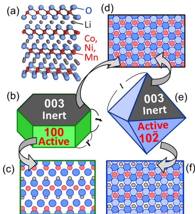
**Fig. 3** (a) Crystal structure of NCM. (b and e) Miller indices of hexagonal plate and octahedral NCM crystals. Atomic arrangements of each crystal facet: (c and f) electrochemically active and (d) inactive surfaces.
