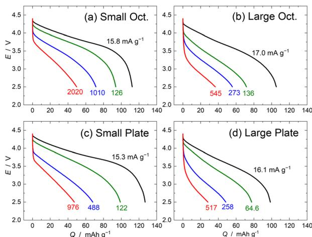
**Fig. 1** Discharge curves during the rate capability tests of diluted NCM electrodes containing 10 wt% NCM. Morphology of NCM: (a) small octahedral, (b) large octahedral, (c) small plate-like, and (d) large plate-like particles.
