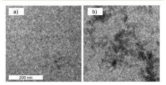
**Fig. 10** Experimental investigation of LLPS in ZIF-8. Cryo-TEM of the solution frozen a) 10 s and b) 60 s after mixing, respectively. Adapted with permission from Liu *et al.*<sup>45</sup> Copyright 2021 National Academy of Sciences. The scale bar applies to both images.
